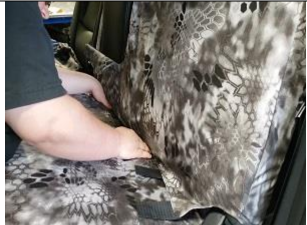
Step 14. Driver & Passenger Top/DT&PT: Tuck the front side in, then fold the backrest down.
