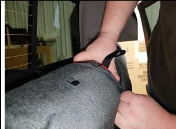
Step 11. Driver Top/DT: Route the tab to release the backrest through the provided hole.
