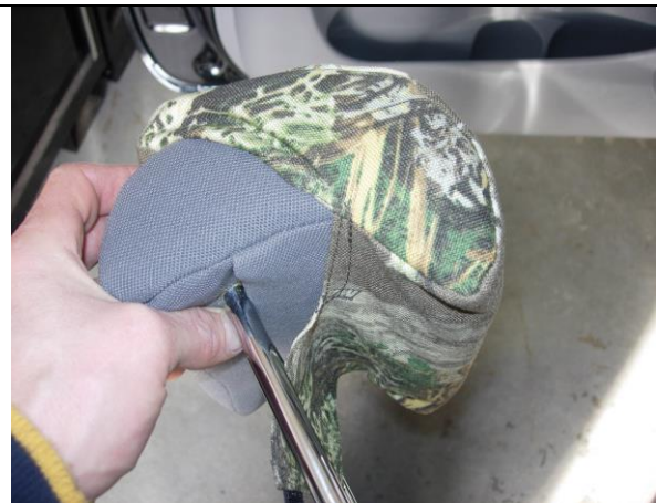
Step 14. Middle Headrest/MH: Slide the cover over the front of the headrest with the extending hook Velcro™ to the front. Connect the Velcro™ same as step 11.
