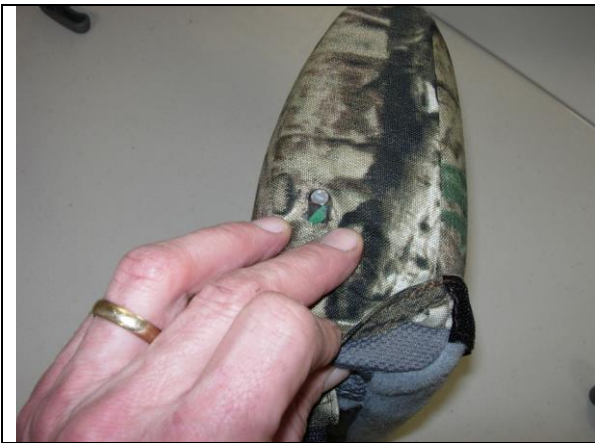
Step 11. Left and Right Headrests/H: Line up the hole in the cover for the lever.
