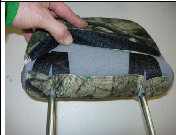
Step 13. Left and Right Headrests/H: Pull the Velcro from the front side around to the back and connect it to the carpet on the back of the headrest, then press the back edge down.
