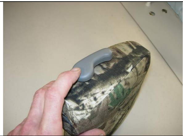
Step 12. Left and Right Headrests/H: Snap the lever back on.
