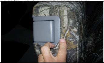
**Step 7. Driver and Passenger Bottoms/DB&PB:** Tuck the fabric under the plastic of the seat release. The fabric only tucks in on the top and ¾ of the way down both sides. Plastic studs close to the edge keep you from tucking it.
