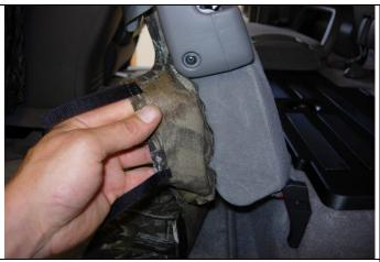
**Step 2. Driver and Passenger Bottoms/DB&PB:**Pull the outside edge of the seat cover around the side of the seat and tuck it behind the plastic.
