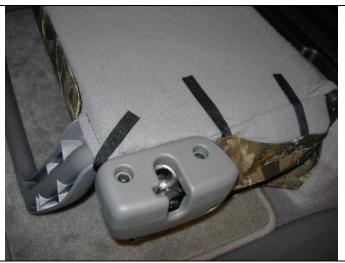
Step 5. Driver and Passenger Bottoms/DB&PB: Mate the two outside edge  $Velcro^{TM}$  to the carpet under the seat.
