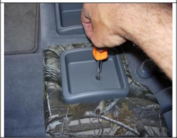
**Step 7. Driver and Passenger Bottoms/DB&PB:**Slide the plastic tongues into the front of the opening and push the tray down into position, and then reinstall the screw.
