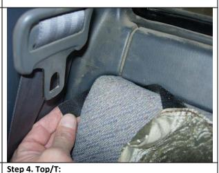
It isn't necessary to remove backrest to install the seat covers. Damage could be done to the clips holding the plastic cowling and be expensive to repair. It may be removed by carefully prying the plastic cowling from under the rear window off, then prying the plastic from the underside of the backrest, then removing the #10 Metric bolts on top and bottom.
