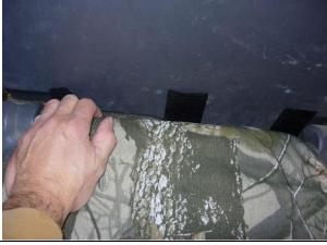
Step 2. Driver & Passenger Bottom/DB&PB: Tuck the Velcro™ into the seat and fold the seat up.
