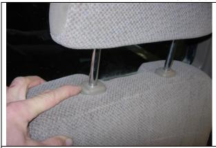
**Step 1. Headrest removal:**Lift the headrests all the way up, then depress the push button release and remove the headrests.
