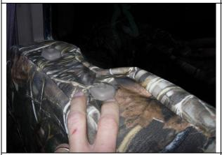
**Step 3. Top/T:**Tuck the fabric under the plastic for the headrests starting with the push button side.
