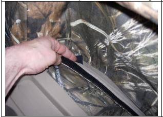
**Step 17.** Armrest/A: Feed the extending hook fasteners through the gap on the left and right side, mating the fasteners in back.
