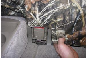
**Step 5. Top/T:**Tuck the bottom of the seat cover in as shown around the seatbelts. Tuck the seat cover between the seat and the silver child restraints leaving them exposed.
