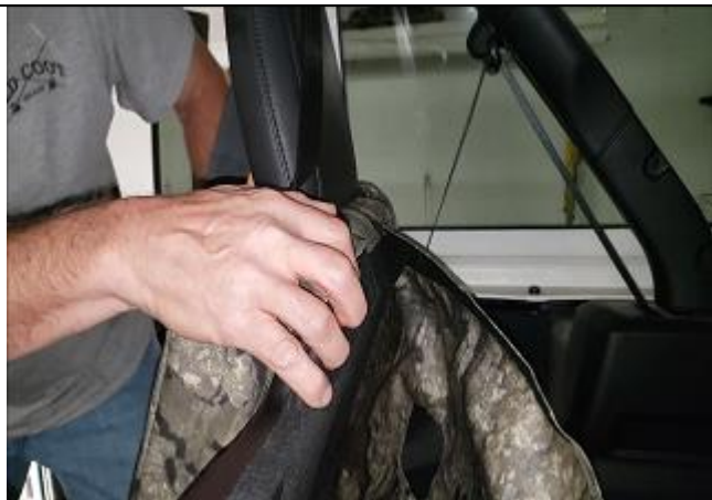
Step 24. PT/Passenger Top: Hold all the Velcro down flat against the back of the seat.
