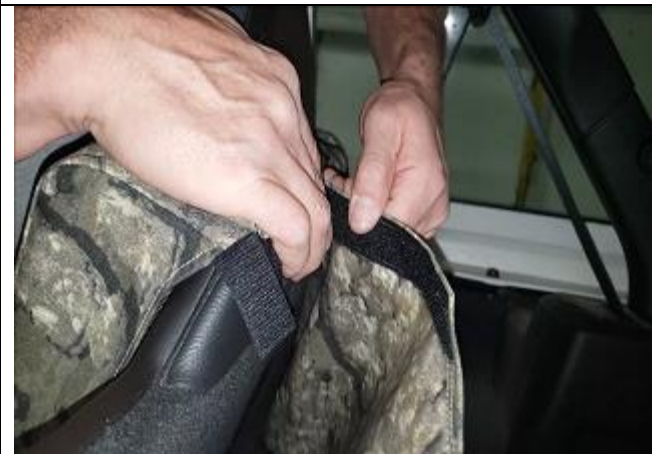
Step 25. PT/Passenger Top: As you hold them down connect the rest of the back flap to the Velcro that is folded over.
