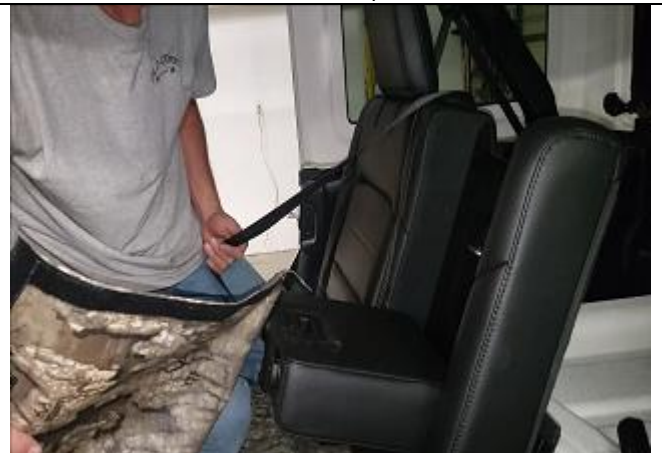
Step 20. PT/Passenger Top: Pull the seatbelt away from the seat and pass the cover under the seatbelt.
