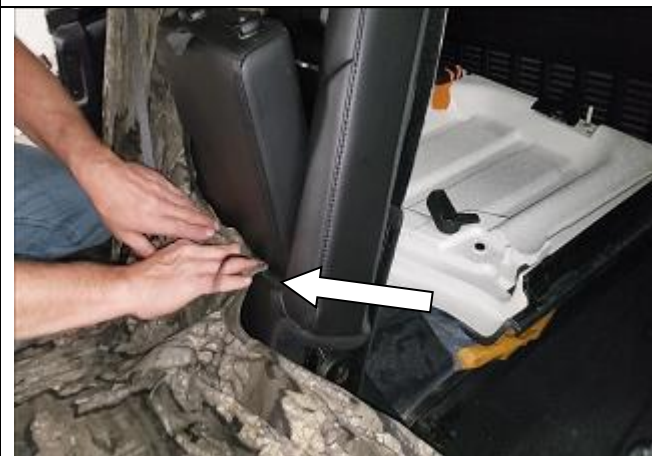
Step 27. PT/Passenger Top: Find the area on the front of the cover with extending Velcro and tuck it under the armrest.
