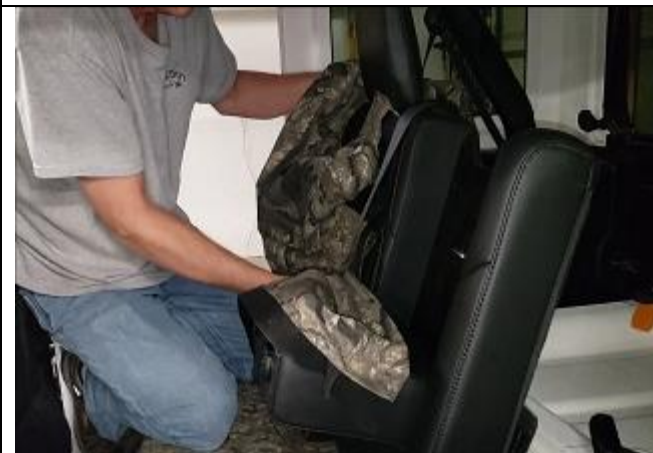
Step 21. PT/Passenger Top: Hook the corner of the cover around the corner of the seat and wrap the cover around the rest of the seat.
