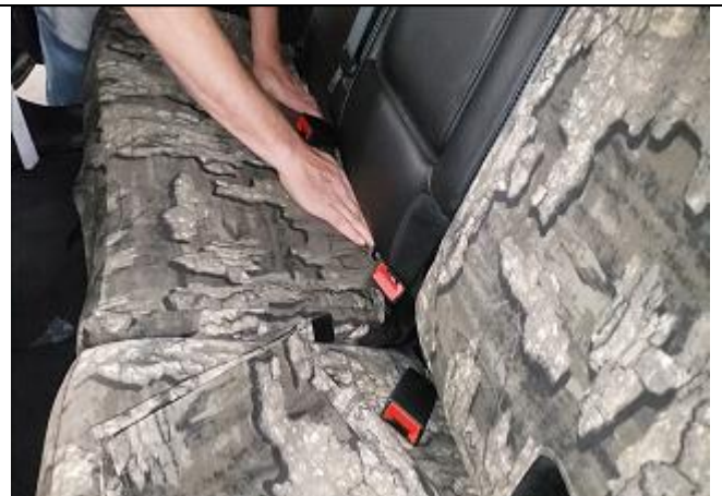
Step 18. PB/Passenger Bottom: The passenger seat installs the same way just bigger and without the seatbelt's elastic strap.
