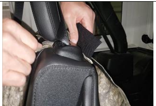
Step 22. PT/Passenger Top: Similar to steps 4 and 5. Feed the front flap under the headrest, pull it tight and connect it to the back flap. You can also tuck the cover under the release levers on the corner of the seat.
