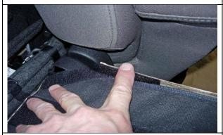
Step 9. Driver & Passenger Top/DT&PT: Connect the outside edge 1"X12" hook Velcro™ to the loop Velcro sewn inside the seat cover on the left and right side.
