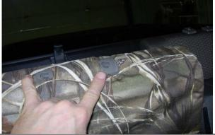
**Step 7. Driver & Passenger Top/DT&PT:**Tuck the seat cover under the plastic for the headrests starting with the push button release.
