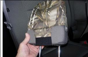
**Step 1. Headrests/H:** All the parts of the seat cover are labeled inside on the bottom right side. Slide the headrest covers on with the extending hook (sticky) Velcro<sup>™</sup> to the front.
