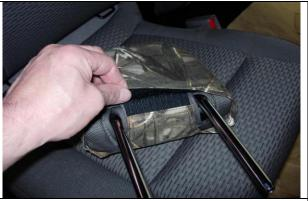
**Step 2. Headrests/H:** Form the cover to the headrest by lining up the seams of the cover to the seams on the headrest, they should closely match.
