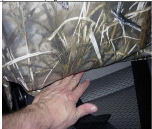
**Step 9. Driver & Passenger Top/DT&PT:** Tuck in the front edge of the seat cover and fold the backrest forward. Make sure to pull the cover down far enough that the rounded bottom left and right corners are forming to the bottom of the backrest.
