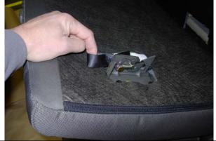
**Step 6. Driver & Passenger Top/DT&PT:** Release the driver side backrest by lifting the seat bottom up all the way. Feel for the nylon webbing pull tab behind the top of driver side down about six inches and pull it up until the seat releases. The passenger side backrest has an exposed nylon release strap that can be seen on Step 11.
