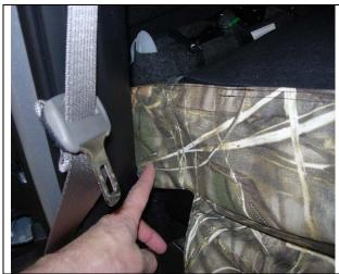
**Step 7. Driver & Passenger Top/DT&PT:** First, slide the seat cover over the outside part of the seat on the outside edge of the seat. This is a flap that hangs down past the pivot point. The seat cover has a pocket that'll slip right over it.
