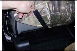
**Step 5. Driver & Passenger Bottoms/DB&PB:** Tuck in the top side, pull it tight and press the hook Velcro<sup>™</sup> to the fuzzy carpet on the back edge of the seat. Lastly pull the bottom side tight and press it to the fuzzy carpet under the seat.
