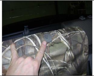
**Step 8. Driver & Passenger Top/DT&PT:** Tuck the seat cover under the plastic for the headrests starting with the push button release.
