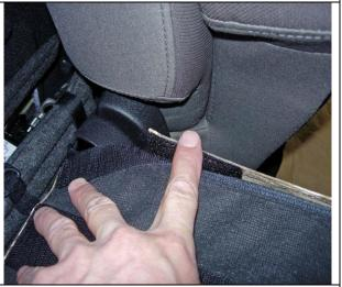
**Step 10. Driver & Passenger Top/DT&PT:** Connect the outside edge 1"X12" hook Velcro™ to the loop Velcro sewn inside the seat cover on the left and right side.
