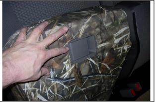
**Step 4. Driver & Passenger Bottoms/DB&PB:** Again, line up the seams of the seat cover to the seams of the seat, and line up the opening for the seat release latch as shown.
