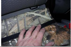
**Step 3. Driver & Passenger Bottoms/DB&PB:** Slide the seat covers on with the letters DB & PB to the top.
