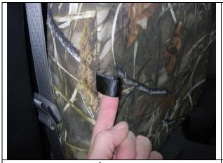
**Step 11. Passenger Top/PT:** Feed the nylon seat release trap through the provided opening.
