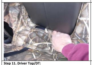
Push the fabric in under the armrest, pressing the hook Velcro™ to the carpet on the back of the armrest cavity, just past the plastic on the bottom.
