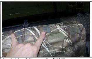
**Step 7. Driver & Passenger Top/DT&PT:**Tuck the seat cover under the plastic for the headrests
