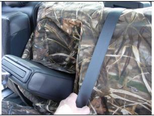
**Step 9. Driver Top/DT:** Tuck the cover behind the seatbelt and poke the armrest through the provided opening.
