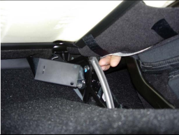
Step 23. Passenger Bottom: Press the Velcro™ to the carpet under the seat.
