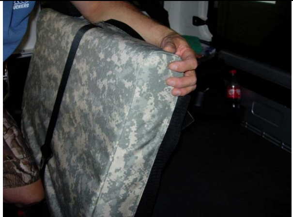
Step 8. Passenger Top/PT: Form the cover over the inside corner. Line up the seams of the seat cover to the seams on the seat, they should match closely.
