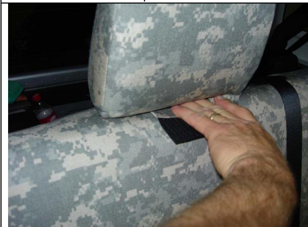
Step 33. Driver Bottom/DB: From under the front of the seat, use the Cordura strap to pull the bungee cord into place and attach it, remove the Cordura strap.
