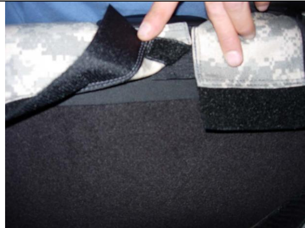
Step 9. Passenger Top/PT: Connect the Velcro™ behind the seatbelt.
