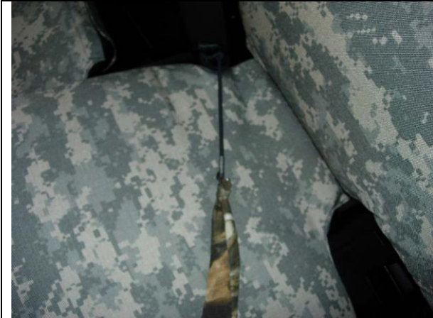
Step 31. Driver Bottom/DB: Tie one of the Cordura straps the cover was sent with to the elastic on the seatbelt.
