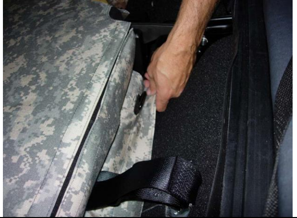
Step 20. Passenger Bottom: As in Step 20, route the metal loop thru the seat cover, then press the Velcro™ to the carpet fuzz on the back edge of the seat.
