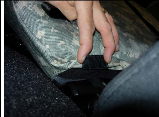
Step 13. Passenger Top/PT: Press the small hook Velcro™ to the carpet fuzz on the outside bottom corner below the nylon pull strap.
