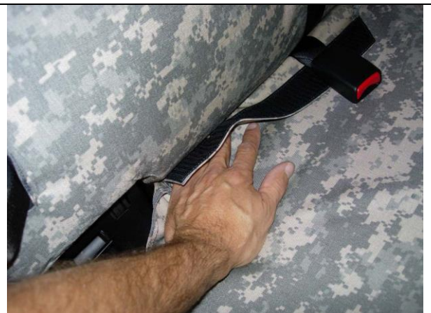
Step 18. Passenger Bottom: Tuck the back edge of the seat cover in.
