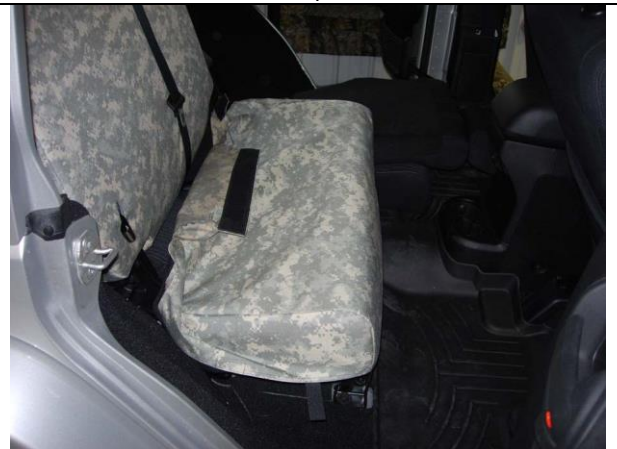
Step 16. Passenger PB/PB: Place the seat cover on as shown, and line up the seams of the seat cover to the seams of the seat.
