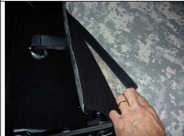
Step 15. Passenger Top/PT: Likewise with the back edge, press it to the carpet.
