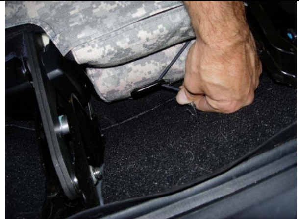
Step 32. Driver Bottom/DB: Re-route the bungee cord thru the metal loop on the back of the seat and tuck the Cordura strap under the seat..
