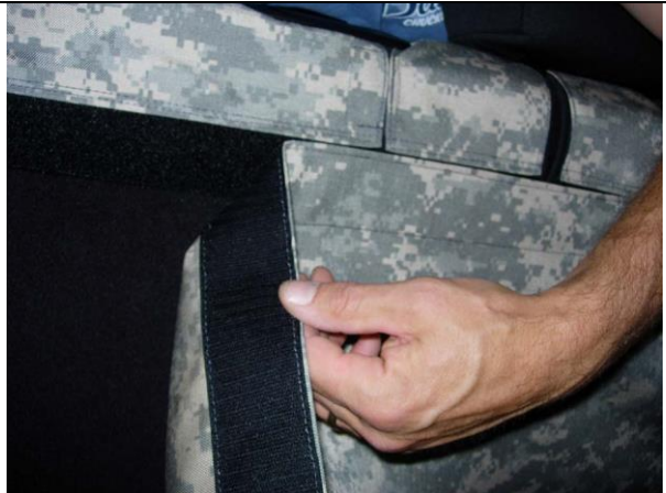
Step 10. Passenger Top/PT: Connect the Velcro™ behind the top of the seat.
