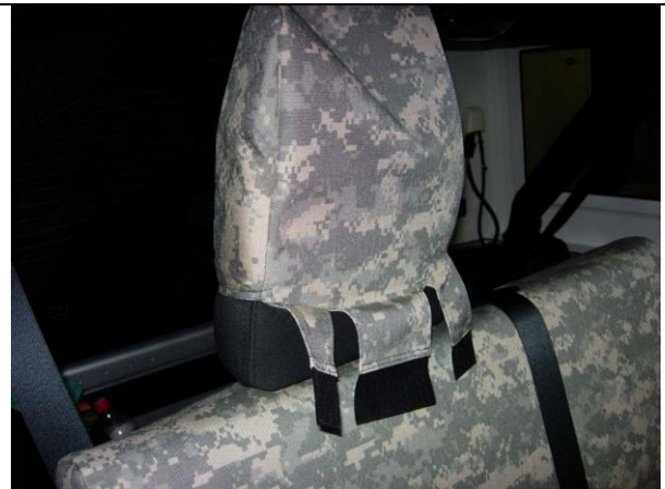
Step 34. Headrests/H: Slide the headrest cover on with the extending Velcro™ to the front, line up the seams.
