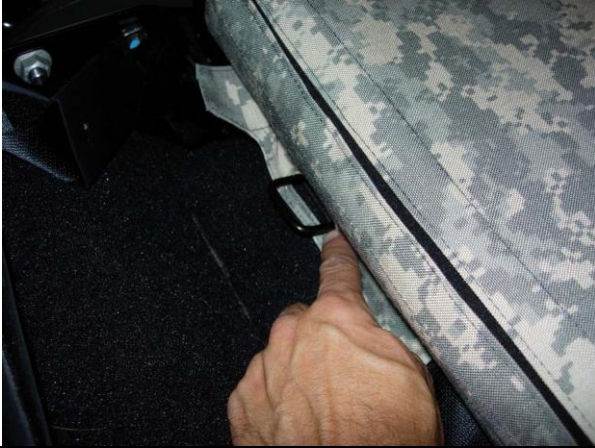
Step 19. Passenger Bottom: Pull the cover back and feed the metal loop thru the seat covers provided opening on the inside edge.
