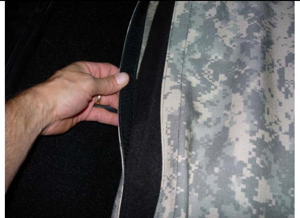
Step 14. Passenger Top/PT: Fold the seat forward and tuck the front edge in. Press the Velcro™ to the carpet on the seat.
