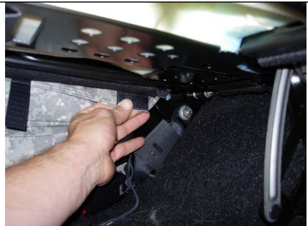
Step 30. Driver Bottom/DB: Place the cover on same as Step 17, press the Velcro™ to the carpet under the seat, and front and back edge.
