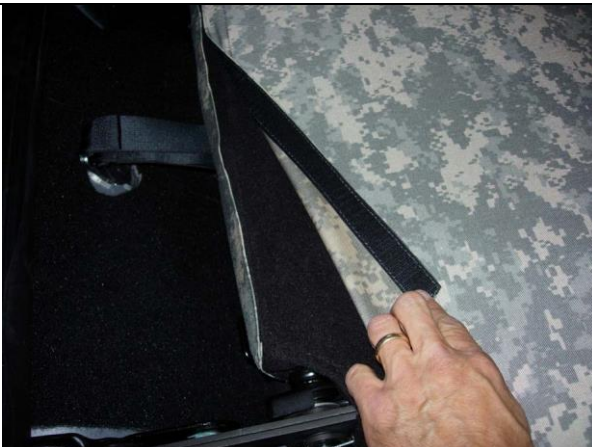
Step 29. Driver Top/DT: Same as Step 15 & 16, connect the Velcro™ to the seat carpet.
