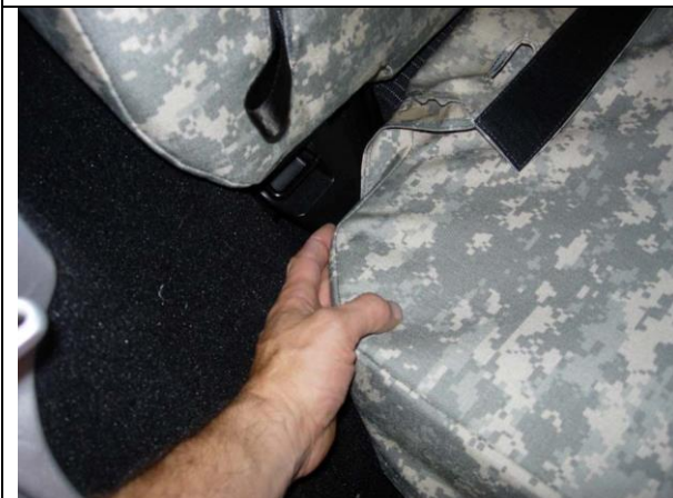
Step 17. Passenger Bottom: Tuck the cover around the back outside corner of the seat.
