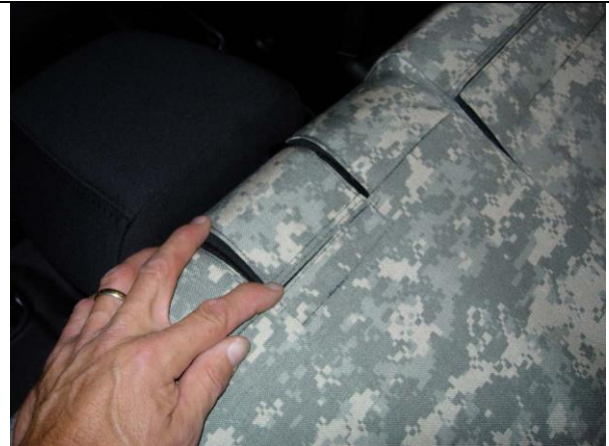
Step 28. Driver Top/DT: As in Step 11, connect the Velcro™ behind the top of the seat.
