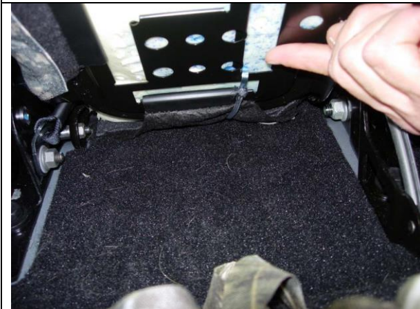
Step 33. Driver Bottom/DB: From under the front of the seat, use the Cordura strap to pull the bungee cord into place and attach it, remove the Cordura strap.
