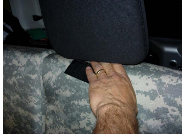
Step 26. Driver Top/DT: Tuck the Velcro™ under the headrest, and tuck the fabric under the plastic for the lever to fold the backrest down.
