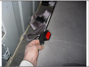
**Step 6. Passenger Bottom/PB:** Remove the seatbelts from their elastic restraints in the middle of the seat.
