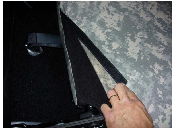
Step 30. Driver Top/DT: Same as Step 15 & 16, connect the Velcro™ to the seat carpet.
