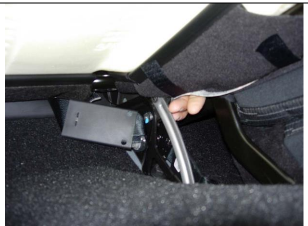
Step 24. Passenger Bottom: Press the Velcro™ to the carpet under the seat.
