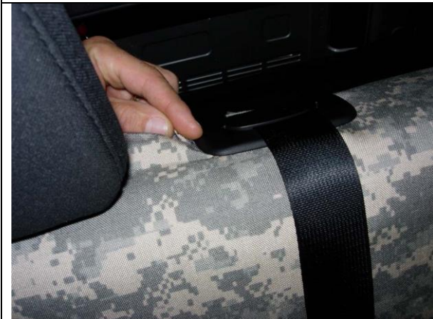
Step 9. Passenger Top/PT: Tuck the fabric under the plastic for the center seatbelt.
