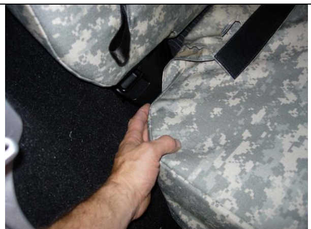
Step 18. Passenger Bottom: Tuck the cover around the back outside corner of the seat.
