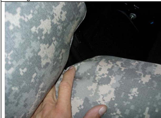
Step 23. Passenger Bottom: Pull the cover around the back inside corner.
