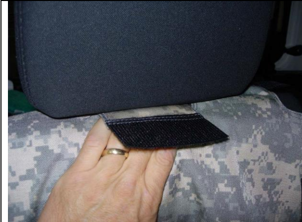
Step 7. Passenger Top/PT: Form the seat cover over the outside corner and tuck the Velcro™ under the headrest.
