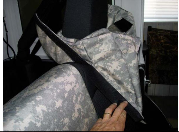
Step 26. Driver Top/DT: Fold the passenger seat down and form the top corners of the seat cover to the seat, lining up the seams.
