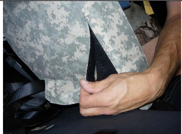
Step 28. Driver Top/DT: Connect the vertical Velcro™ on the inside edge.
