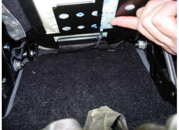
Step 34. Driver Bottom/DB: From under the front of the seat, use the Cordura strap to pull the bungee cord into place and attach it, remove the Cordura strap.
