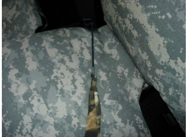
Step 32. Driver Bottom/DB: Tie one of the Cordura straps the cover was sent with to the elastic on the seatbelt.
