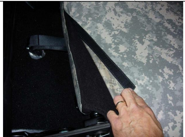
Step 16. Passenger Top/PT: Likewise with the back edge, press it to the carpet.
