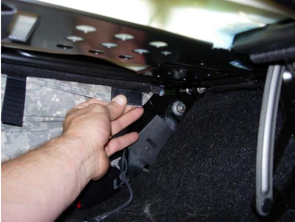
Step 31. Driver Bottom/DB: Place the cover on same as Step 17, press the Velcro™ to the carpet under the seat, and front and back edge.
