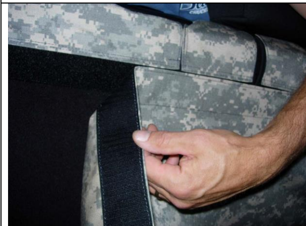
Step 11. Passenger Top/PT: Connect the Velcro™ behind the top of the seat.
