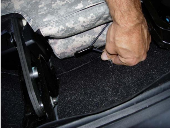
Step 33. Driver Bottom/DB: Re-route the bungee cord thru the metal loop on the back of the seat and tuck the Cordura strap under the seat..
