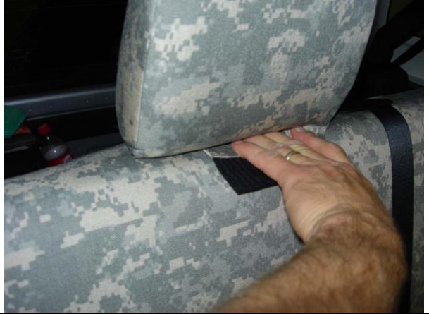
36. Headrests/H: Tuck it under the headrest and connect it to the loop Velcro™ sewn inside the back edge.
