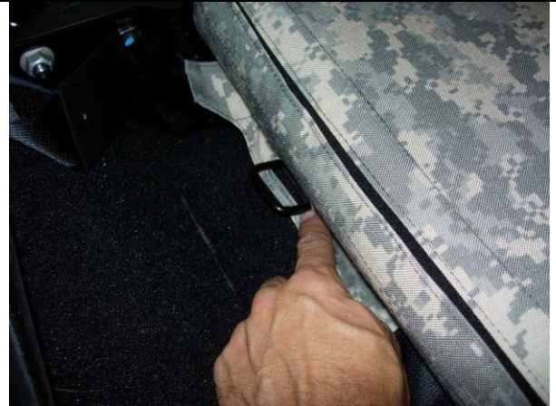
Step 20. Passenger Bottom: Pull the cover back and feed the metal loop thru the seat covers provided opening on the inside edge.
