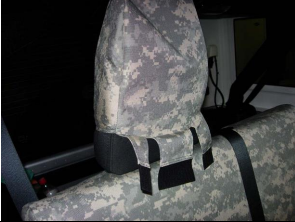
35. Headrests/H: Slide the headrest cover on with the extending Velcro™ to the front, line up the seams.
