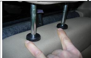
**Step 1. Top/T:** Remove the headrests by lifting them up all the way using the push button release on the right side. Next, use gentle upward pressure and depress the semihidden push button release on the left.
