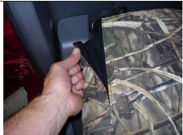
Step 10. Driver & Passenger Bottom/DB&PB: Lastly, pull the cover tight and press the remaining Velcro™ to the fuzz.
