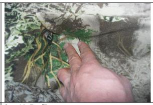
**Step 14. Top/T:**If there is fuzzy carpet on the back of the armrest cavity, mate the two hook fasteners sewn inside the corners of the seat cover to the carpet.
