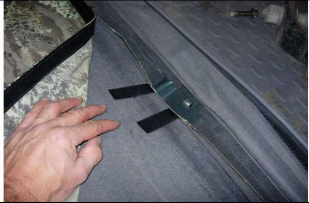
Step 14. Driver and Passenger Top/DT&PT: Pull the hook Velcro™ in front of the seat belt tight and press them to the carpet on the seat back.
