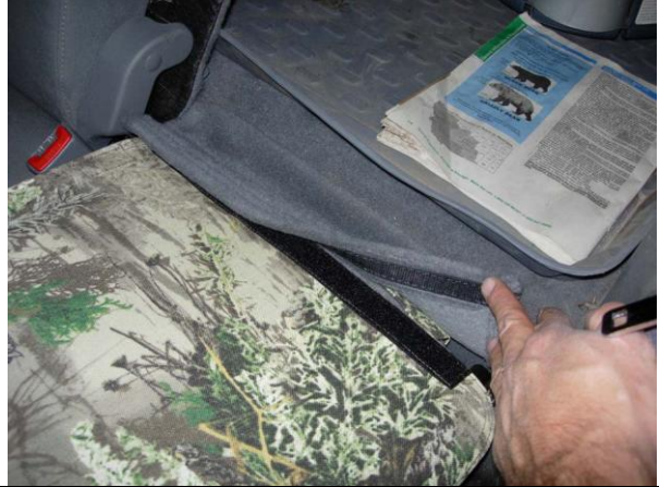
Step 16. Driver and Passenger Top/DT&PT: Reconnect the carpeted flap to the loop Velcro™ sewn on the outside of the seat cover.
