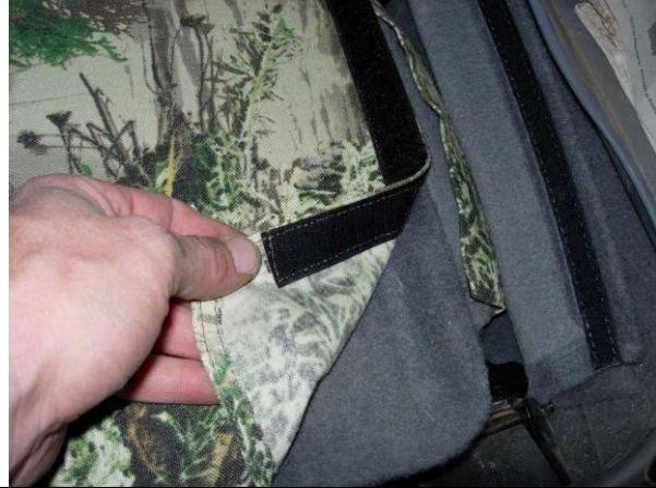
Step 15. Driver and Passenger Top/DT&PT: Press the back edge of the seat cover to the carpet on the seat back
