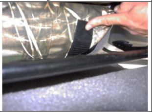
Step 12. Driver and Passenger Bottom/DB&PB: Pull the back edge of the seat cover back and press it to the carpet on the back edge. Using one hand in a smoothing action from front to back helps remove the slack and tighten the cover.
