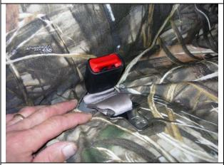
**Step 9. Driver Bottom/DB:** Feed the seat belts through he provided opening.
