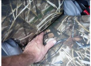
**Step 10. Driver and Passenger Bottom/DB&PB:** Tuck the back edge of the seat cover in.
