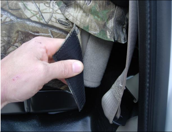
Step 5. Bottom: Pull the sides back and connect the hook Velcro™ to the carpet on the seat as shown.
