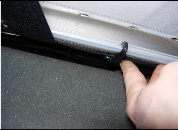
Step 9. Bottom: From under the front of the seat, reach in and clip the no-slip hooks over the plastic. From behind the seat connect the hook Velcro™ to the rear loop Velcro™. Trim the excess length of all the Velcro™.
