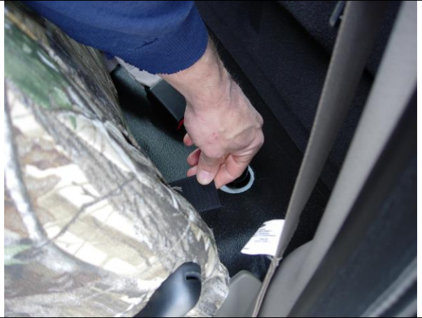
Step 6. Bottom: Route the long hook Velcro™ under the front of the seat and connect them to the loop Velcro™ sewn on the back edge.
