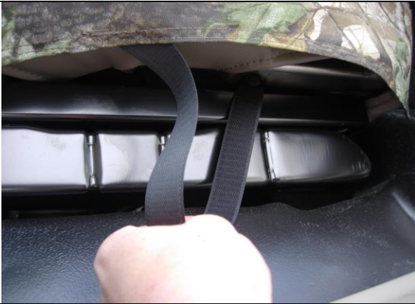
Step 7. Bottom: Route the long side hook Velcro™ over the top of the metal frame and connect them to the loop Velcro™ on the back edge at an angle, trim off the excess.
