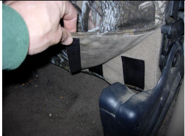
Step 8. Driver & Passenger Bottom/DB & PB: Press the hook Velcro™ on the bottom side to the carpet as shown.
