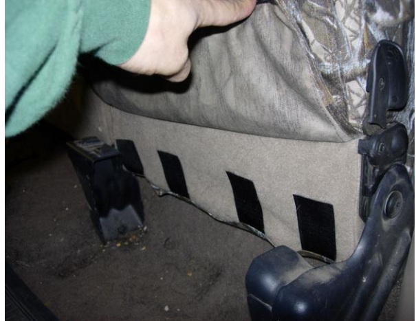
Step 6. Driver & Passenger Bottom/DB & PB: Slide the covers on with the extending hook Velcro™ to the top side, pressing them to the carpet as shown.
