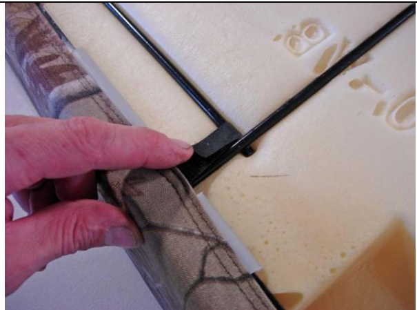
Step 16. Bottom/B: Press it onto the hook Velcro™. Check to see if all the holes for mounting the metal seat back are aligned.
