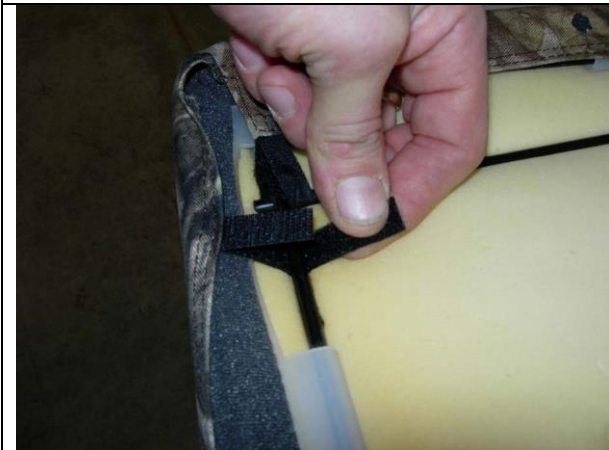
Step 17. Bottom/B: Connect the sides by sliding the loop Velcro™ under the metal bar.
