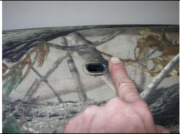
Step 14. Bottom/B: Place the Bottom on and position the opening for the seat release strap, and turn the seat upside down. Same as Step 8, align the holes for mounting the metal seat back.
