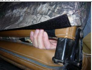
**Step 4. Top/T:** Tuck the Velcro<sup>™</sup> into the seat. Use one hand in a smoothing action down the front of the seat cover while gently pulling on the Velcro<sup>™</sup> from the backside with the other hand. Use the front hand to pin the Velcro<sup>™</sup> to the seat, then press the Velcro<sup>™</sup> together. Work your way across from one side to the other.
