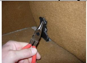
**Step 1. Seat Preparation:** Fold the seat forward and remove the pins on left and right as shown. Slide the whole seat to the right and remove it. Place it on a table for an easier installation.
