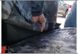
**Step 15. Driver & Passenger Top/DT&PT:**Recline the backrest, and grab the front of the seat cover as shown, pulling it down hard in the area where the big hook Velcro™ is sewn on.
