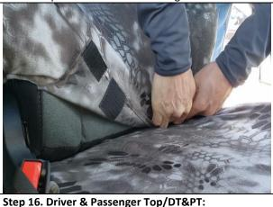
While holding the seat cover tight. First press the two big hook Velcro™ to the fuzzy carpet on the front edge, then press the two small outside Velcro™ to the fuzzy carpet. You may have to reconnect the Velcro™ for the best fit.
