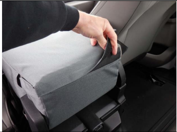
Step 28. Armrest/A: Connect the far back Velcro™.
