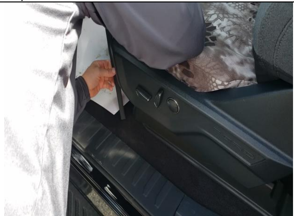
Step 10. Driver & Passenger Bottom/DB&PB: Run the Velcro under the seat. Make sure you don't bind any wires. The Velcro™ needs to go above any wires that are dangling down.
