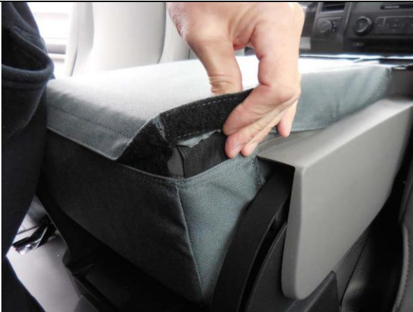
Step 29. Armrest/A: Connect the right side Velcro™
