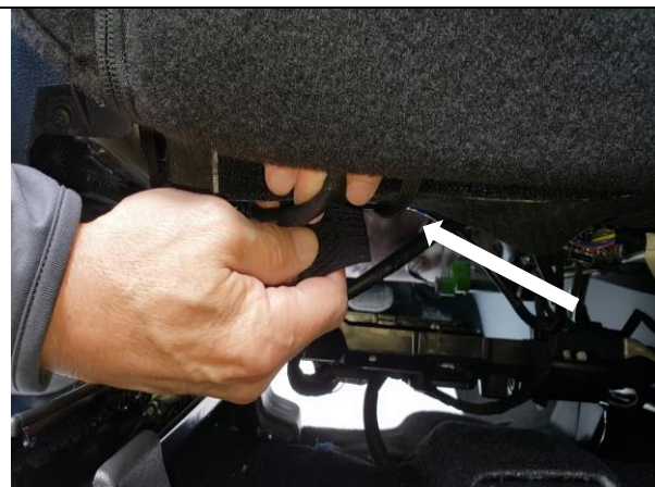
Step 11. Driver & Passenger Bottom/DB&PB: Pull the carpeted panel away from the back edge of the seat and connect the front hook Velcro™ to the loop (fuzzy) Velcro™ in back, making sure they connect on the far left and right side of the back edge.
