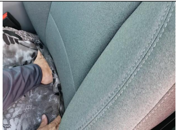
Step 8. Driver & Passenger Bottom/DB&PB: Line up the front seam, and left and right. Once everything looks good, tuck in the back edge all the way.
