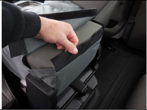
Step 26. Armrest/A: Pull the bottom edge up from the backside.
