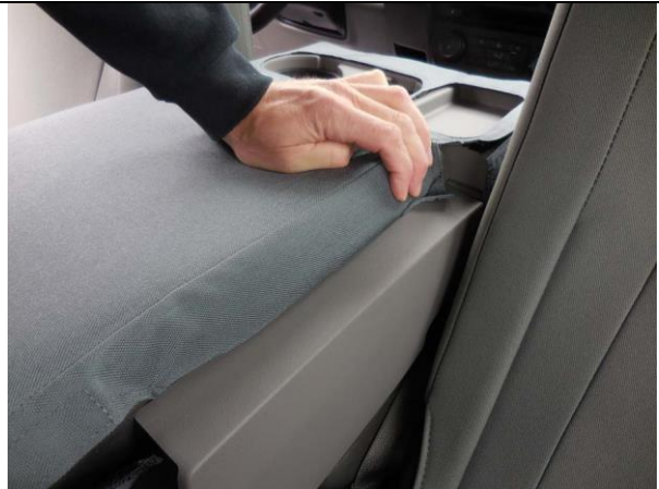
Step 30. Armrest/A: Lastly, tuck the fabric behind the plastic as shown.
