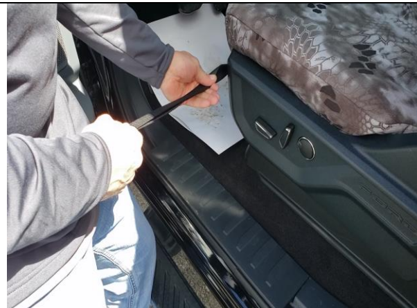
Step 9. Driver & Passenger Bottom/DB&PB: If you have electric seats be sure to lift the seat up as high as it will go. This will pull everything away from your seat and free up some space. Fold the long front hook Velcro™ in half lengthwise with the sticky facing in. This will stiffen the Velcro™ and make it easier to run under the seat.
