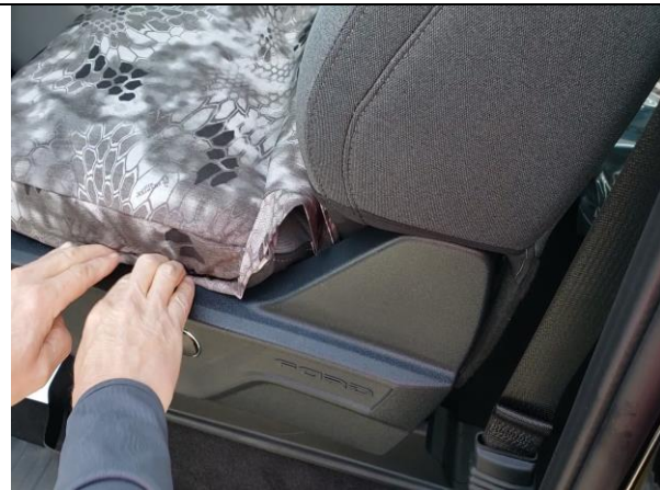
Step 7. Driver & Passenger Bottom/DB&PB: Take the outside edge of the cover and tuck it behind the plastic.
