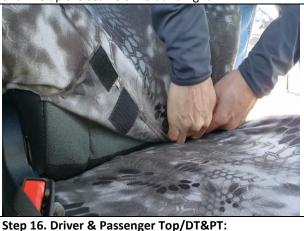
While holding the seat cover tight. First press the two big hook Velcro™ to the fuzzy carpet on the front edge, then press the two small outside Velcro™ to the fuzzy carpet. You may have to reconnect the Velcro™ for the best fit.
