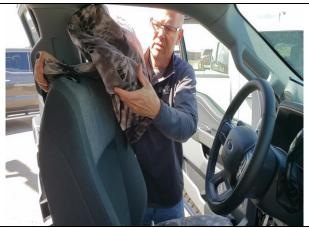
**Step 13. Driver & Passenger Top/DT&PT:**Slide the seat cover on with the abbreviations DT & PT to the front side.
