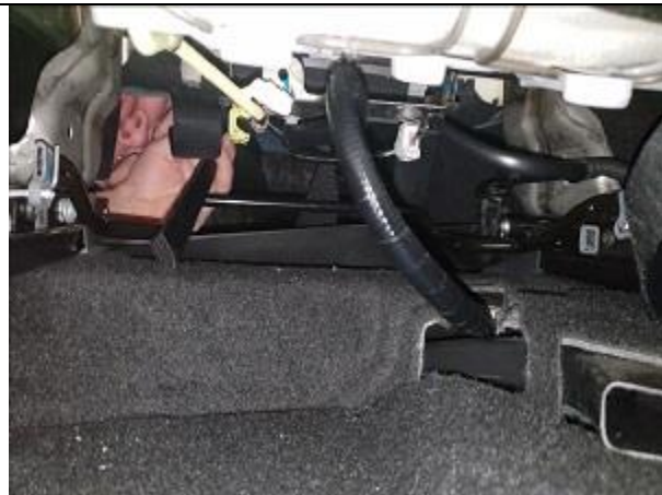
Step 13. Driver & Passenger Bottom/DB&PB: Make sure the Velcro is above any wires or bars that are hanging loose and are not tightly bound to the seat already.
