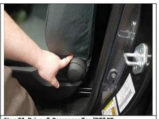
**Step 22. Driver & Passenger Top/DT&PT:**Tuck the seat cover behind the plastic molding on the outsides of the seat.
