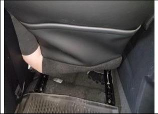
**Step 14. Driver & Passenger Bottom/DB&PB:**Connect the Velcro™ from the front to the loop Velcro™ sewn on the back edge.
