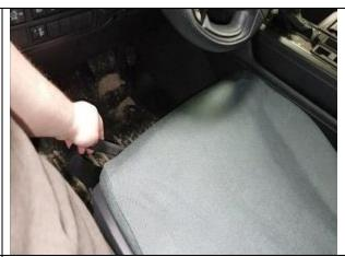
**Step 12. Driver & Passenger Bottom/DB&PB:**Fold the long front hook Velcro™ in half lengthwise.
