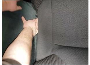
Step 11. Driver & Passenger Bottom/DB&PB: Tuck the back edge of the seat cover into the seat. From behind the seat, pull the cover back hard, forming it to the front of the seat.
