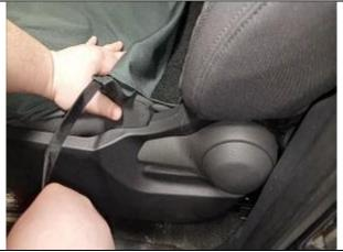
**Step 7. Driver & Passenger Bottom/DB&PB:**Fold the outside edge Velcro™ in half lengthwise with the sticky facing in. This stiffens it, making it easier to route.
