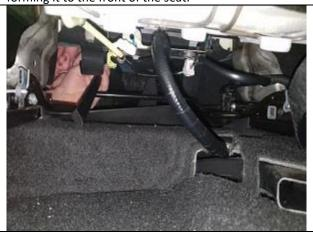
Step 13. Driver & Passenger Bottom/DB&PB: Route the Velcro™ above wires or metal framework, keeping it directly under the seat.
