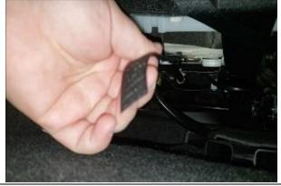
Step 16. Driver & Passenger Bottom/DB&PB: (This is a picture of a truck that has a removable flap.) This is what your Velcro should look like under the flap.
