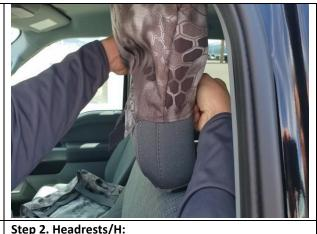
All the parts of the seat cover are labeled inside. Use the Seat Cover Part ID chart to ID parts. Slide the headrest covers on with the extending hook (sticky) Velcro™ to the front.
