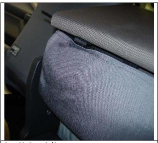
**Step 23. Console/C:**Disconnect the adhesive Velcro<sup>™</sup> from the two inside back edge loop Velcro<sup>™</sup>. With the console down, slide the Velcro thru the gaps in the hinge.
