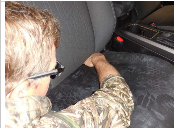
Step 15. Driver & Passenger Bottom/DB&PB: Connect the inside edge Velcro same as Step 12.
