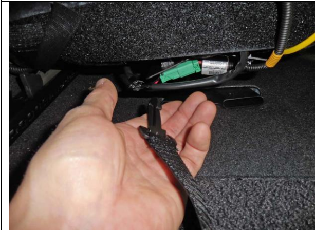
Step 17. Driver & Passenger Bottom/DB&PB: The two plastic buckles connect under the back edge of the seat about 6-8" apart.
