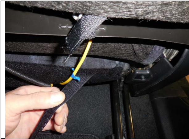
Step 13. Driver Bottom/DB: Route the hook Velcro™ around the back corner and press it to the loop Velcro™
