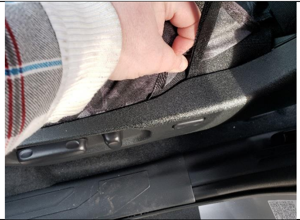
Step 14. Driver Bottom/DB: Fold the Velcro™ in half same as Step 8, and route the outside Velcro in-between the seat and plastic. There will be a small hole where shown. Route same as Step 12 & 13.
