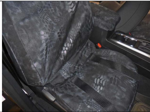
Step 27. Driver & Passenger Top/DT&PT: Slide the seat all the way forward, then slide the covers on with the extending hook Velcro™ to the front.
