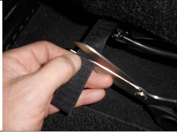
Step 25. Driver & Passenger Bottom/DB&PB: Again, trim the excess length.
