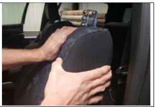
**Step 12. Driver & Passenger Top/DT&PT:** Form the top of the seat cover to the top of the seat. Next, line up the seams of the seat cover to the seams of the seat on left and right, they should match closely.
