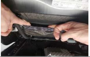
**Step 16. Driver & Passenger Top/DT&PT:** Next, wrap the material around the metal bar.
