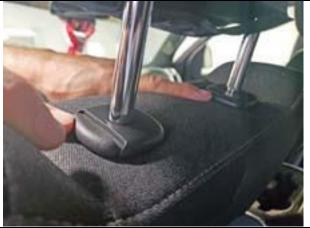
**Step 2. Headrests/H:** Recline the seats so the headrest will clear the roof while removing it. Release the headrests by gently lifting them up all the way. Then, depress the two buttons at the same time
