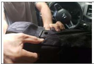
Step 11. Driver & Passenger Top/DT&PT: Provisions are made for the side impact airbags. It is critical to get the covers on the correct side. The covers are marked on the inside front right "DT & PT" for Driver & Passenger Top. Also note, the Driver Top has our Headwaters Seat Cover label on the backside.
