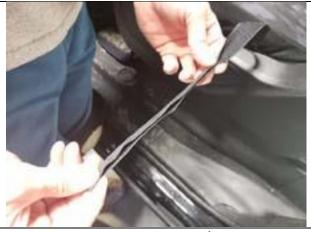
**Step 24. Driver & Passenger Bottom/DB&PB:** Again, for electric controlled seats, lift the seat/seats all the way up. This clears a path to route the Velcro<sup>™</sup>. Fold the side Velcro<sup>™</sup> in half lengthwise as shown, with the sticky facing in. This will make it stiff and easier to route.
