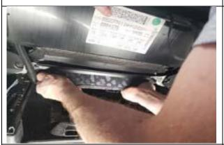
**Step 15. Driver & Passenger Top/DT&PT:** Pull the material tight with both hands. Then use one hand in a smoothing action down the front of the seat cover from top to bottom, while pulling on the cover from behind the seat with the other hand to gain slack on the front side.
