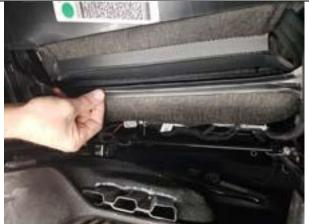
**Step 10. Seat Preparation** Carefully press the tape to the metal bar.
