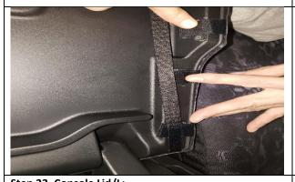
**Step 33. Console Lid/L:** Lastly, fold the side Velcro<sup>™</sup> under the lid to see where they'll lay. Prepare the areas with rubbing alcohol by scrubbing hard, then wiping them dry while wet. If the adhesive Velcro<sup>™</sup> are not sticking, re-clean the areas with warm to hot soapy water and rag. Then reclean areas with rubbing alcohol.
