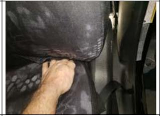
**Step 22. Driver & Passenger Bottom/DB&PB:** Tuck the back edge in carefully under the metal bar. From behind, pull the cover back and tight to the front of the seat as shown on Step 23.
