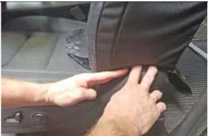
**Step 13. Driver & Passenger Top/DT&PT:** Tuck in the outsides of the seat cover behind the plastic molding as shown
