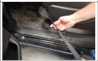
**Step 27. Driver & Passenger Bottom/DB&PB:** Same as Step 24, fold the long front of the seat hook Velcro<sup>™</sup> in half lengthwise with the sticky facing in.
