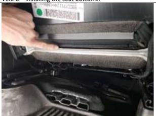
**Step 8. Seat Preparation** Next, locate the metal bar at the back edge of the seat. This bar is super sharp on top and bottom and capable cutting your seat cover.
