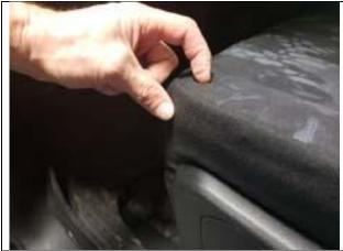
**Step 23. Driver & Passenger Bottom/DB&PB:** Same as Step 12, line up the seams of the seat cover to the seams of the seat along the sides and front. Work the material inside the cover outward, or from forefinger to thumb.
