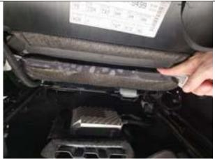
**Step 19. Driver & Passenger Top/DT&PT:** Pull the other side tight and connect same as Step 16. Look at the front side and see if the cover is fitting snug. If not, repeat Step 15 to snug the cover.
