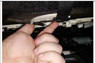
**Step 30. Driver & Passenger Bottom/DB&PB:** Connect the two plastic buckles under the backside of the seat to the frame. Position them left and right, centered with about 6-8" between them.
