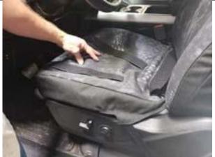
**Step 21. Driver & Passenger Bottom/DB&PB:** Place the cover on with the long hook Velcro<sup>™</sup> to the front as shown. Use caution working under the seat. All the metal is razor sharp, and anything that moves has grease. Look at your hands before touching the seat cover after working under the seat to avoid getting grease on to your seat cover. Keep a paper towel or rag handy.
