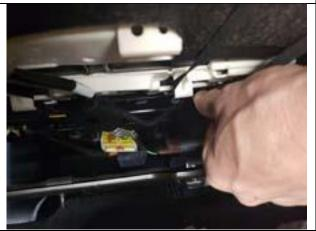
**Step 7. Seat Preparation** Follow the elastic under the seat to where it's connected, and push it forward to release it.
