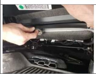
**Step 9. Seat Preparation:** Cover the top and bottom edge with electrical tape, or use 2" wide tape and do in one shot.
