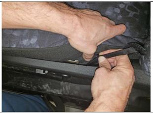
**Step 25. Driver & Passenger Bottom/DB&PB:** Slide the side Velcro<sup>™</sup> straight down from where it's sewn on.
