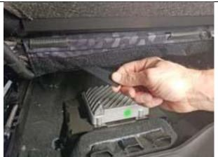
Step 26. Driver & Passenger Bottom/DB&PB: Use a light when working under the seat. Locate the side Velcro<sup>™</sup>, and route it thru the gap in the frame to the back corner, avoid wires. Similar to Step 15, slide your hand down the outside edge of the cover while gently pulling on the Velcro<sup>™</sup>, then press it to the loop Velcro<sup>™</sup> sewn on the back edge as shown. Be careful to not over tighten and create wrinkles.
