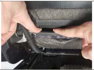
**Step 18. Driver & Passenger Top/DT&PT:** Press the provided "pinch welt" over the material onto the metal bar.
