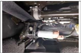
**Step 29. Driver & Passenger Bottom/DB&PB:** Same as Step 28, route the front Velcro<sup>™</sup> where shown, avoiding the mechanisms and wiring.
