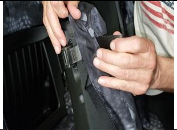
Step 26. DTS&PTS/Driver & Passenger Top Storage: Covers for the Driver Top Storage & Passenger Top Storage are labeled inside the bottom right of each part. "DTS & PTS". Feed the storage compartment release strap thru the provided opening.
