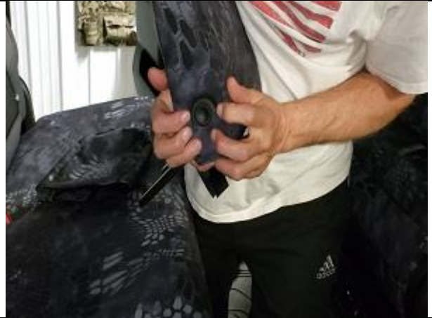
Step 8. H/Headrest: Tuck the fabric behind the plastic for the push button. Lastly, connect the Velcro™.
