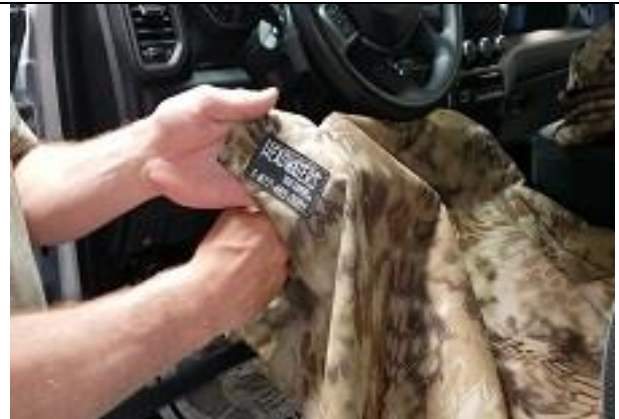
Step 17. Driver & Passenger Top/DT&PT: Provisions are made for the side impact airbags. It is critical to get the covers on the correct side. The covers are marked on the inside front right "DT & PT" for Driver & Passenger Top. Also note, the Driver Top has our Headwaters Seat Cover label on the backside.
