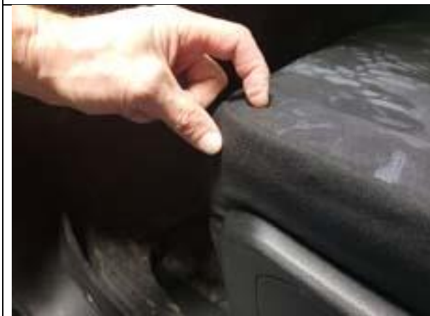
Step 35. Driver & Passenger Bottom/DB&PB: Same as Step 24, line up the seams of the seat cover to the seams of the seat along the sides and front. Work the material inside the cover outward, or forefinger to thumb.
