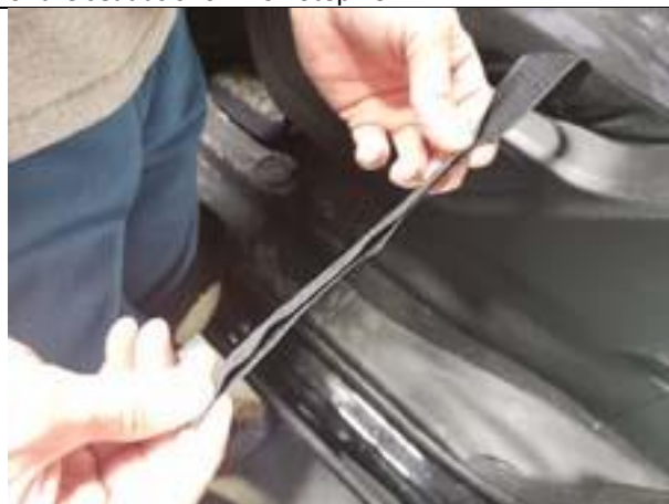
Step 36. Driver & Passenger Bottom/DB&PB: Electric seats, lift the seat up as high as possible. Fold the side hook Velcro™ in half lengthwise as shown, with the sticky facing in. This will stiffen it, making it easier to route.
