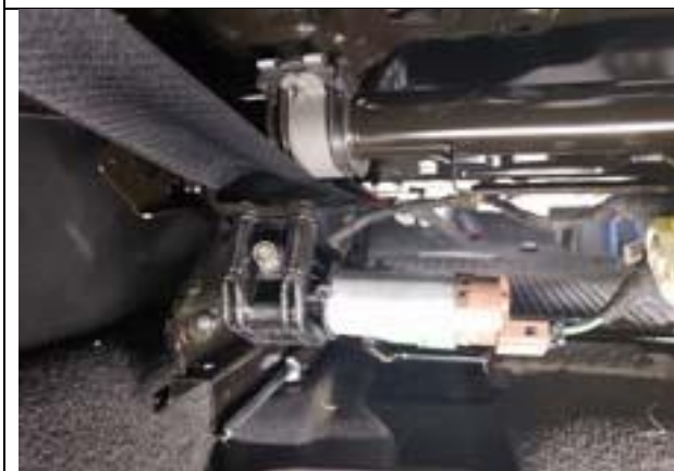
Step 41. Driver & Passenger Bottom/DB&PB: Same as Step 28, route the front Velcro™ where shown, avoiding the mechanisms and wiring.
