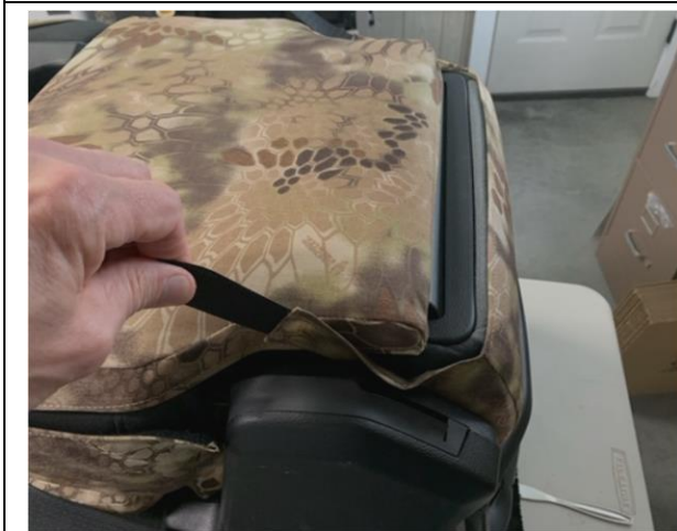
Step 11. Console/C: Pull the left and right back corners up and around the hinge area.
