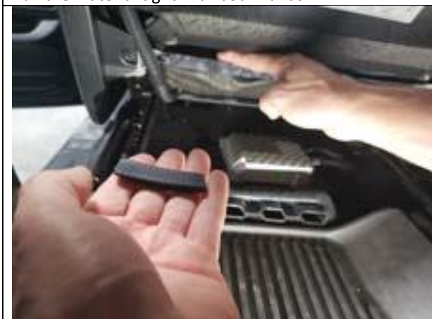
Step 29. Driver & Passenger Top/DT&PT: Start on one side. Hold the material tight with one hand.
