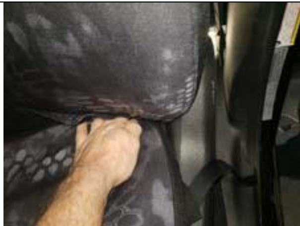
Step 34. Driver & Passenger Bottom/DB&PB: Tuck the back edge in carefully under the metal bar. From behind, pull the cover back and tight to the front of the seat as shown on Step 23.
