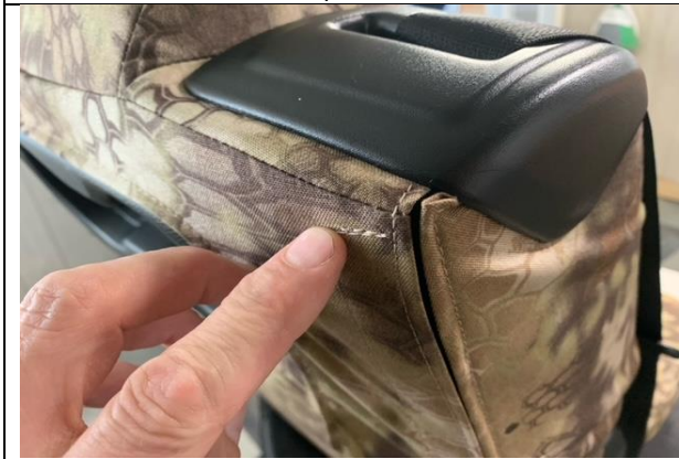
Step 9. Console/C: Tuck the fabric on the right side up under the plastic as far as you can, then temporarily connect the Velcro™
