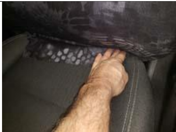
Step 26. Driver & Passenger Top/DT&PT: Next, pull down on the front of the seat cover, and carefully tuck it in under the taped up metal bar.
