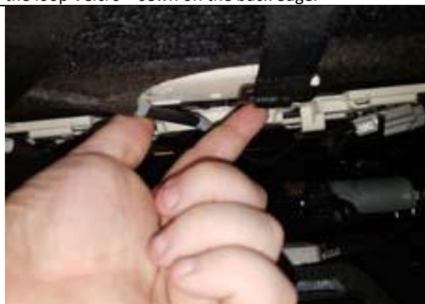
Step 42. Driver & Passenger Bottom/DB&PB: Connect the two plastic buckles under the backside of the seat to the frame, centered with about 6-8" apart. Press them to the loop Velcro™ on the back edge. This is critical to keep the seat anchored in place.
