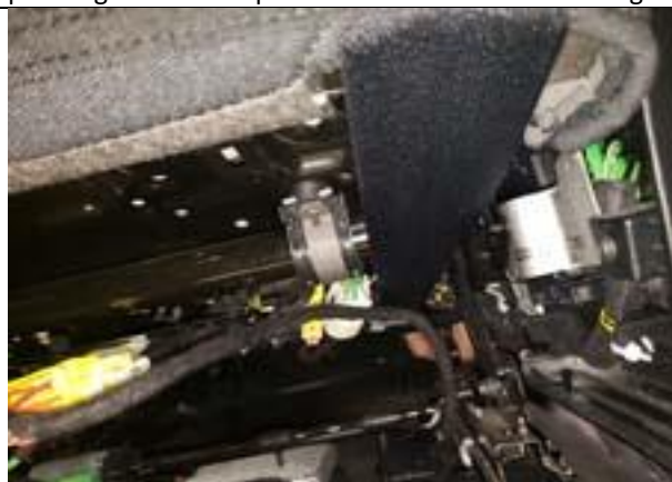
Step 40. Driver & Passenger Bottom/DB&PB: Route the outside front Velcro™ where shown to the back, avoiding any mechanisms or wiring. Connect it to the loop Velcro™ sewn on the back edge.
