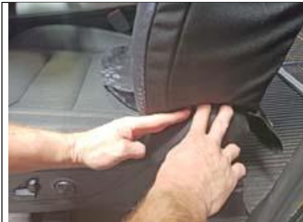
Step 25. Driver & Passenger Top/DT&PT: Tuck the sides behind the plastic as shown.
