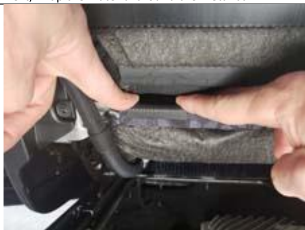
Step 30. Driver & Passenger Top/DT&PT: Press the provided "pinch welt" over the material onto the metal bar.
