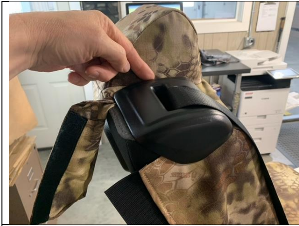
Step 7. Console/C: Form the cover to the integral headrest, then tuck the fabric under the seatbelt plastic where shown.
