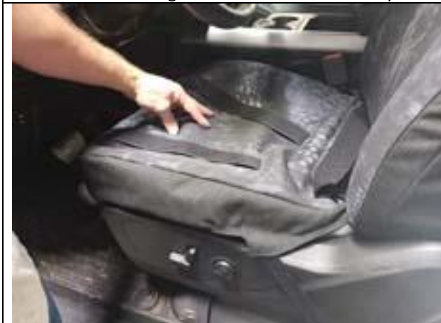
Step 33. Driver & Passenger Bottom/DB&PB: Place the cover on with the long hook Velcro™ to the front as shown.
