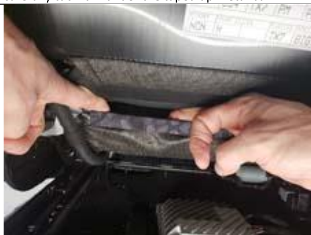
Step 28. Driver & Passenger Top/DT&PT: Next, wrap the material around the metal bar.
