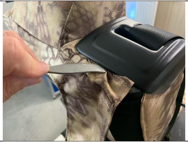
Step 8. Console/C: Continue tucking the fabric under the plastic using a dull butter knife
