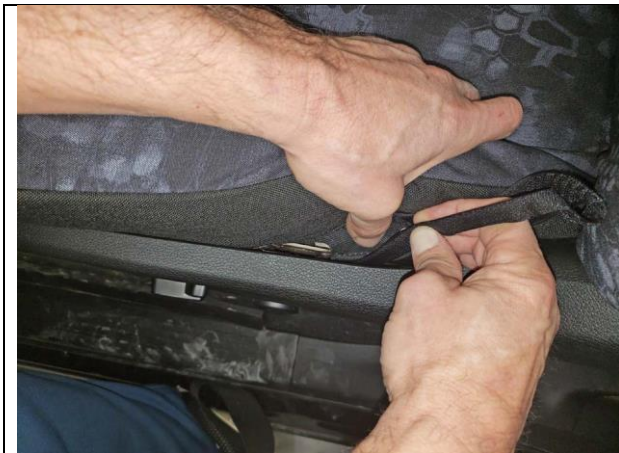
Step 37. Driver & Passenger Bottom/DB&PB: Slide the side Velcro™ straight down from where its sewn on, push about 6-8" in.
