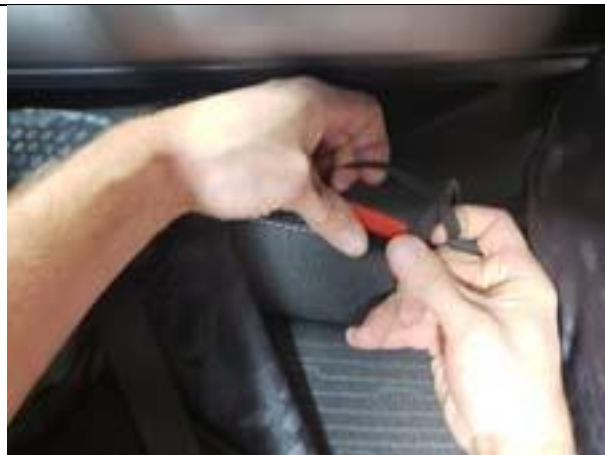
Step 32. Driver & Passenger Top/DT&PT: Remove the seat belt from the elastic as shown.
