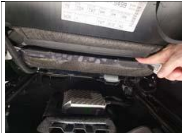
Step 31. Driver & Passenger Top/DT&PT: Pull the other side tight and connect same as Step 16.
