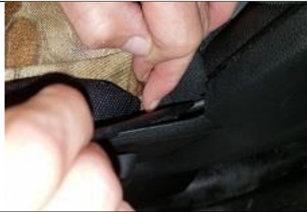
Step 15. Driver & Passenger Bottom: DB/PB Close up view of the driver's seat plastic molding. Fold the long hook (sticky) Velcro™ on the outside edge and fold it in half lengthwise with the sticky facing in. This stiffens it up making it easier to route. Push the seat in and away from the plastic, and push the Velcro™ straight down from where it's sewn on.
