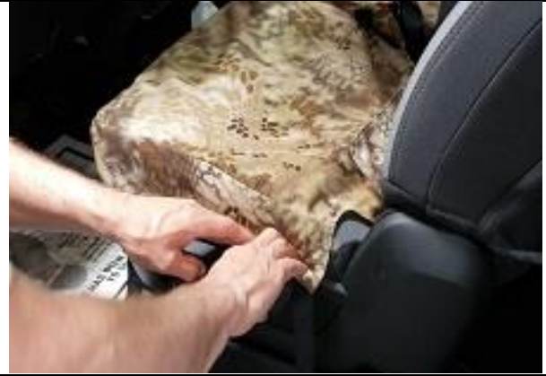
Step 14. Driver & Passenger Bottom: DB/PB DB & PB are printed on the inside right back corner. View of the Driver Seat. Slide the seat forward, and for electric controlled seats, lift the seat all the way up. Carefully disconnect the Velcro™, placing the cover on the seat. Then tuck the back edge, and the outside edge in. From behind the seat, pull on the back edge to help form the seat cover to the front of the seat. Use one hand in a smoothing action from front to back on the seating area while pulling with the other hand from behind the seat.
