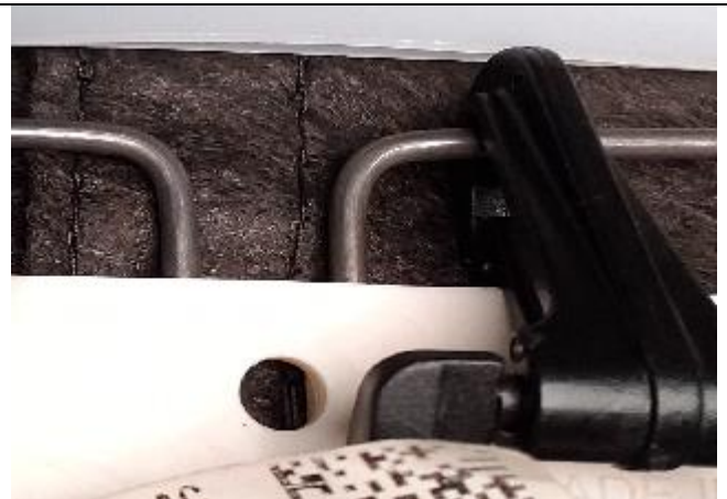
Step 16. Driver & Passenger Bottoms/DB&PB: Take the buckles from earlier and clip them onto the metal bars under the seat. Hook them around the bars toward the center of the seat. Then pull them tight and connect them to the flap.
