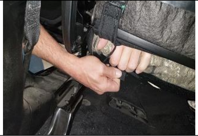
Step 12. Driver & Passenger Bottoms/DB&PB: Pull the seat cover tight and connect the front Velcro to the flap.
