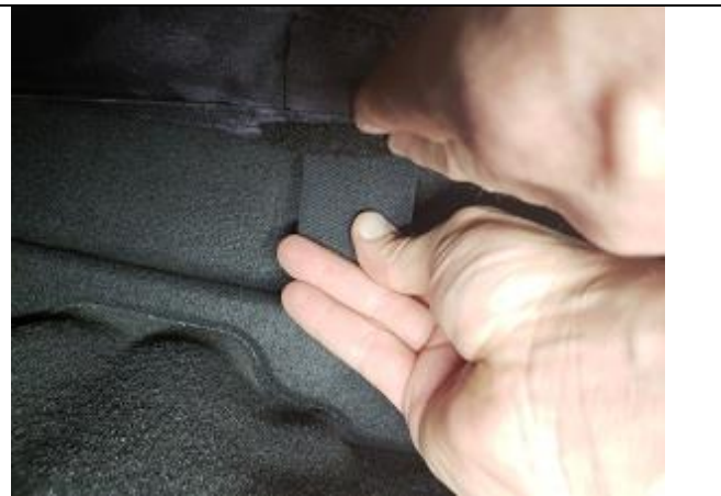
Step 12. DT: Driver Top Reach up behind the seat and feel for the Velcro™ from the top. Pull the down and connect them to the Loop Velcro™ sewn inside the front edge of the seat cover.
