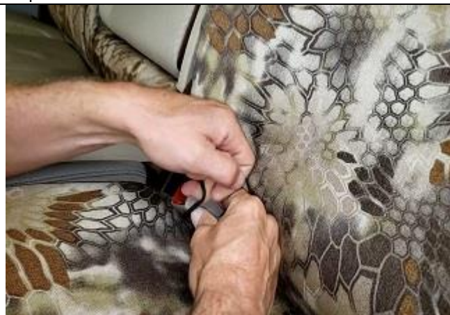
Step 27. DB/PB: Driver and Passenger Bottoms Slide the seatbelts back into the elastic.
