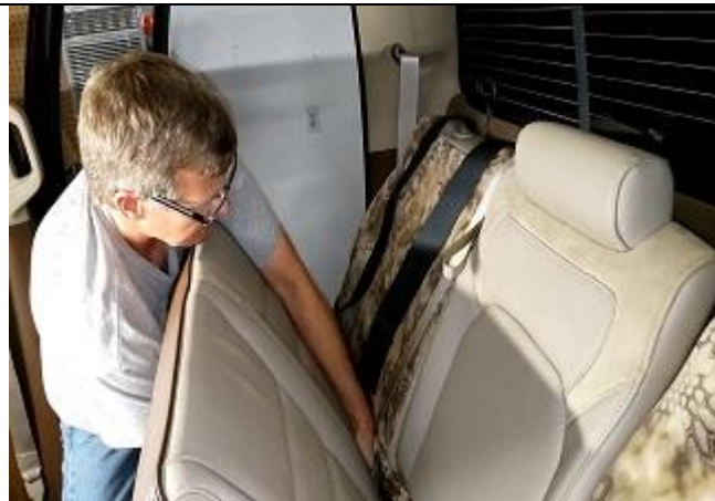
Step 17. PT: Passenger Top With the seat bottom partway up, tuck in the front edge of the seat cover.
