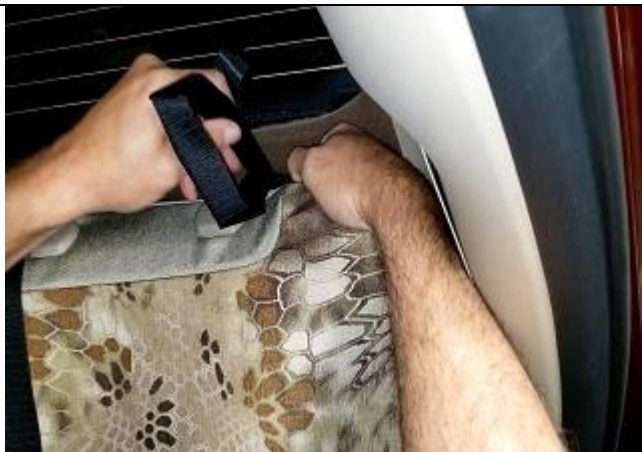
Step 11. DT: Driver Top Lifting the seat bottoms up will pull the top of the seat away from the cab allowing room to route the Velcro™. Fold the 2"x24" Hook Velcro™ in half lengthwise with the sticky facing in. Now it'll be 1"x24" and rigid. Push the Velcro™ straight down.
