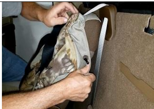
Step 14. PT: Passenger Top Pull the cover over the seat starting with the metal peg that the console latches to.
