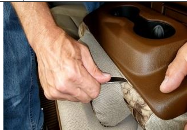
Step 30. C: Console Tuck the cover under the front of the console as shown using the same toothless butter knife.
