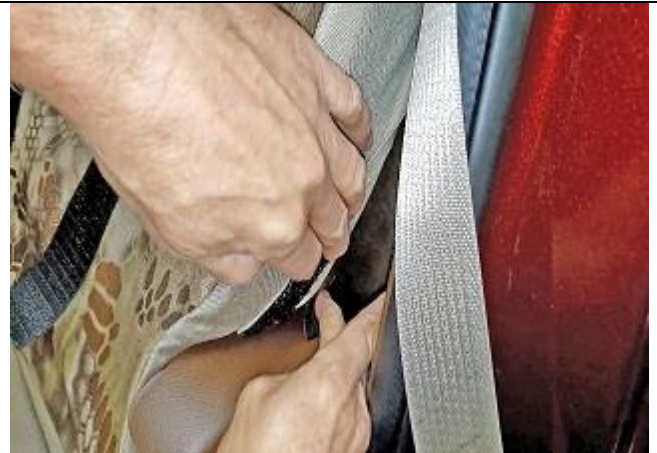
Step 10. DT: Driver Top Route the 1X14 Hook Velcro™ around to the sides of the seat, connecting them to the Loop Velcro™ sewn inside the sides.
