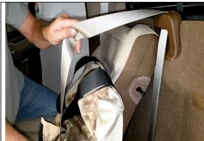
Step 13. PT: Passenger Top Pull the shoulder seatbelt out of the way.
