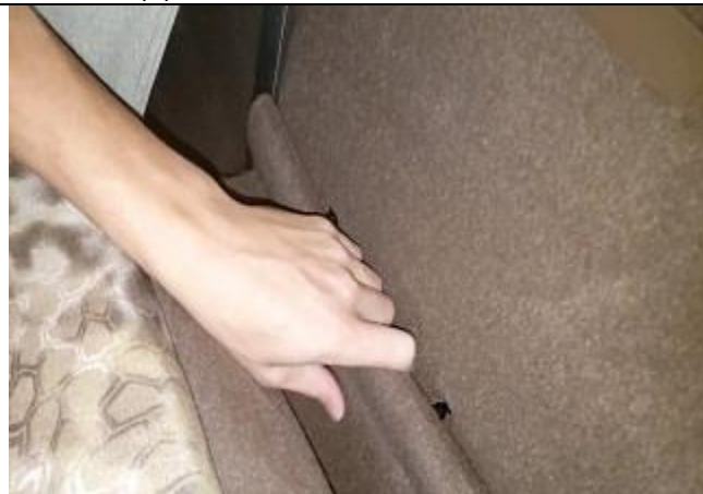
Step 18. PT: Passenger Top Now, fold the console down and look behind it. You'll find a magnetic carpeted flap. Pop the flap off and fold it back.
