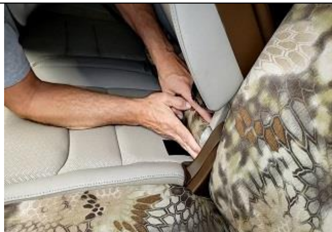
Step 15. PT: Passenger Top Tuck the front of the cover under the seat as shown.
