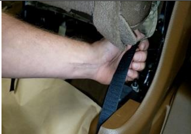
Step 9. DT: Driver Top Locate the Hook Velcro™ front the front side and pull them down. Next, pull the seat cover down forcibly, tightening the front of the seat cover.
