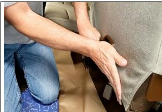
Step 25. DB/PB: Driver and Passenger Bottoms Press the Hook Velcro™ sewn inside the seat cover to the carpet under the seat.
