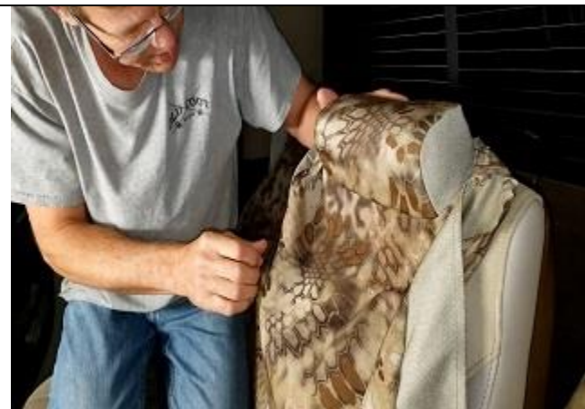
Step 28. C: Console Fold the console forward slightly and pull the cover over the top.
