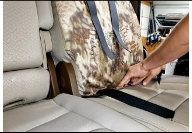
Step 8. DT: Driver Top Tuck in the front edge, along with the 1"x14" hook Velcro™ sewn on left and right.
