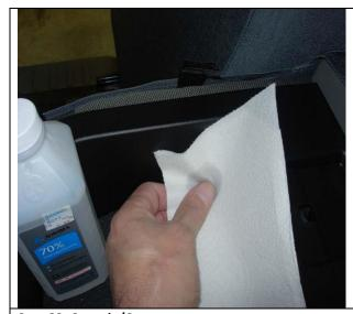
**Step 23. Console/C:** Fold the Velcro<sup>™</sup> into the storage area and see where they will lay. Prepare these areas with rubbing alcohol by scrubbing the area hard, and wipe it dry while it's still wet. With the adhesive Velcro<sup>™</sup> connected to the loop Velcro<sup>™</sup>, remove the backing from the adhesive, pull it snug and press the adhesive Velcro<sup>™</sup> hard into the plastic. See Step 26 for a picture of the rear center Velcro<sup>™</sup> connection.
