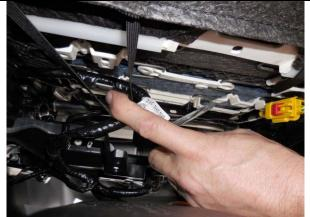
**Step 2. Prepare the seats for installation.** FOR MANUAL SEATS ONLY, disconnect the inside elastic (next to the console) holding the flap under the back edge of the seat. The other one is blocked by an electrical plug. All seats with electric controls, the elastic will not remove because of the electrical plug.
