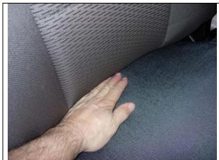
Step 7. Driver & Passenger Bottom/DB&PB: Tuck in the back edge all the way. Line up the front seam, and left and right, then grab the material from behind the seat and pull it down. This will be a little tough on electric controlled seats because the elastic for the panel won't remove.
