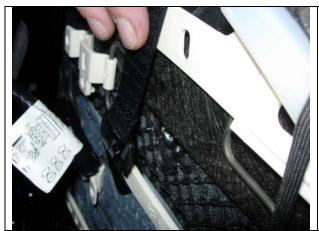
**Step 13. Driver & Passenger Bottom/DB&PB:** Sideways view of under the back edge of the seat. Connect the two plastic buckles where shown to the plastic brace, then connect them to the loop Velcro on the back edge. This will hold the seat cover in place.
