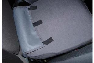
**Step 18. Middle Bottom/MB:** Place the cover on with the three extending hook Velcro<sup>™</sup> to the back. Line up the seams on the front and sides, then flip up the seat and tuck in the back edge.
