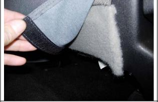
**Step 17. Driver & Passenger Top/DT&PT:** Reconnect the elastic under the seat, then pull the seat cover down in back, pressing the hook Velcro<sup>™</sup> onto the fuzzy carpet on the back edge of the seat.
