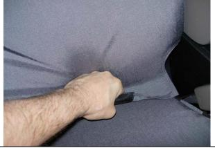
**Step 15. Driver & Passenger Top/DT&PT:** Recline the backrest, and grab the front of the seat cover as shown, pulling it down hard in the area where the big hook Velcro<sup>™</sup> is sewn on.
