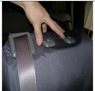
**Step 20. Console/C:** Tuck the fabric under the plastic for the headrests.
