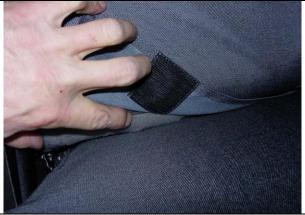
**Step 16. Driver & Passenger Top/DT&PT:** While holding the seat cover tight. First press the two big hook Velcro<sup>™</sup> to the fuzzy carpet on the front edge, then press the two small outside Velcro<sup>™</sup> to the fuzzy carpet. You may have to reconnect the Velcro<sup>™</sup> for the best fit.
