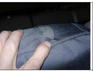
**Step 14. Driver & Passenger Top/DT&PT:** Slide the seat cover on with the abbreviations DT & PT to the front side. Tuck the fabric under the plastic for the headrests. Form the top of the seat cover to the top of the seat and line up the seams on left and right.
