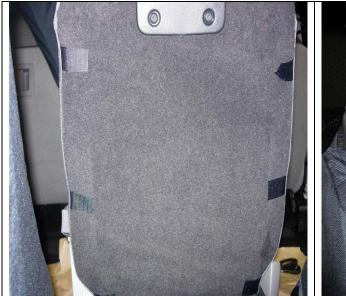
**Step 19. Middle Bottom/MB:** Press the hook Velcro<sup>™</sup> to the fuzzy carpet under the seat as shown.
