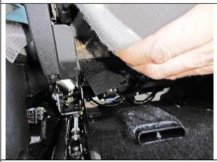
Step 9. Driver & Passenger Bottom/DB&PB: Pull the carpeted panel away from the back edge of the seat and connect the front hook Velcro<sup>™</sup> to the loop (fuzzy) Velcro<sup>™</sup> in back. Make sure the Velcro<sup>™</sup> connect to the far left and right side of the back edge. Avoid pressing wires or electrical plugs under Velcro<sup>™</sup>.
