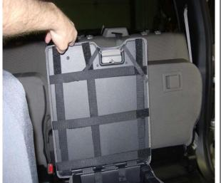
**Step 26. Lid/L:** Connect the Velcro<sup>™</sup> under the lid as shown. Notice the two 1/2" hook Velcro<sup>™</sup> connected at an angle to the loop Velcro<sup>™</sup>.
