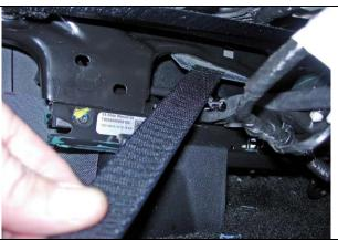
**Step 12. Driver & Passenger Bottom/DB&PB:** Same as Step 12, fold the inside edge Velcro<sup>™</sup> next to the console in half lengthwise and feed it thru the gap as shown. Connect it to the loop Velcro<sup>™</sup> in back at an angle.
