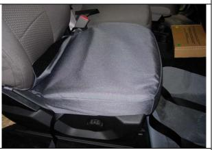
**Step 6. Driver & Passenger Bottom/DB&PB:** Remove the plastic buckles from the back edge of the seat cover and slide the covers on with the extending hook Velcro<sup>™</sup> to the front.
