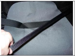
**Step 8. Driver & Passenger Bottom/DB&PB:** If you have electric seats be sure to lift the seat up as high as it will go. This will pull everything away from your seat and free up some space. Fold the long front hook Velcro<sup>™</sup> in half lengthwise with the sticky facing in. This will stiffen the Velcro<sup>™</sup> and make it easier to run under the seat.
