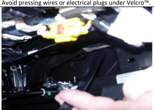
**Step 11. Driver & Passenger Bottom/DB&PB:** View from behind the seat. Look for the Velcro<sup>™</sup> from under the back edge of the seat. Route it thru the gap as shown and connect it to the loop Velcro<sup>™</sup> strip in back at an angle.
