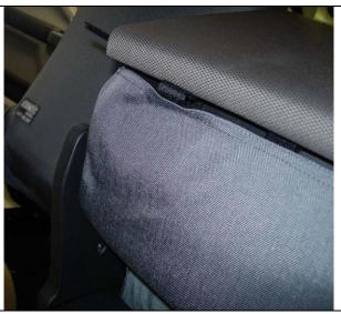
**Step 22. Console/C:** Disconnect the adhesive Velcro<sup>™</sup> from the two inside back edge loop Velcro<sup>™</sup>. With the console down, slide the Velcro thru the gaps in the hinge.
