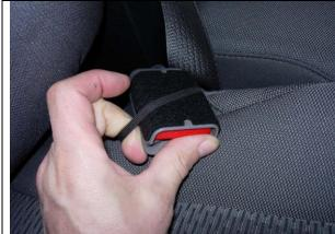
**Step 1.** Prepare the seats for installation. Push the seatbelts located on the inside next to the console thru the elastic on the seat. Lift electric controlled seats all the way up, and then slide the seats forward.
