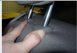
**Step 5. Prepare the Console for installation.** Remove the middle headrest by pushing the two push button releases shown and lift up. It will be a tight squeeze to get your fingers in to do this.
