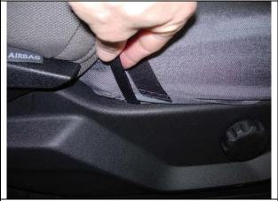
**Step 10. Driver & Passenger Bottom/DB&PB:** Same as Step 8, fold the side hook Velcro<sup>™</sup> in half lengthwise with the sticky facing in. Slide it down exactly where shown.
