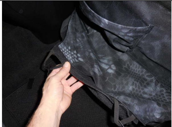
Step 30. Driver & Passenger Top/DT&PT: Press the hook Velcro™ sewn inside the back edge to the carpeted flap behind the seat.
