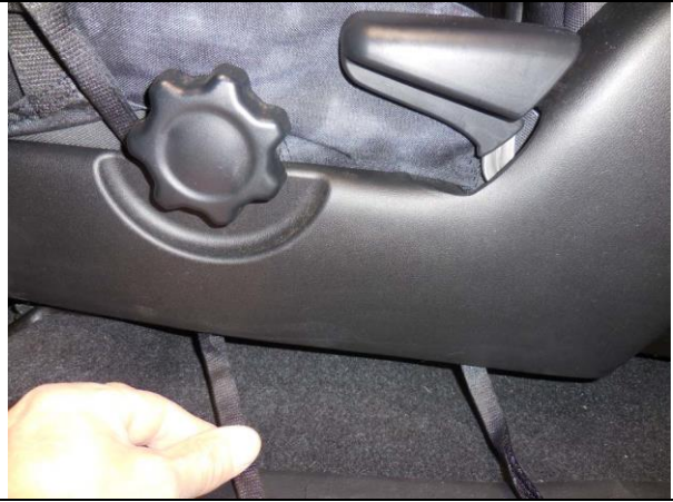
Step 14. Driver & Passenger Bottom/DB&PB: Fold the Velcro™ in half same as Step 8, and route the front Velcro in front of the lumbar knob, route same as Step 12 & 13.
