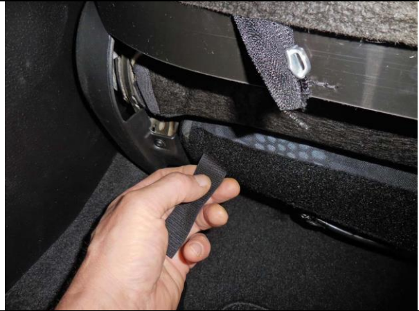
Step 16. Driver & Passenger Bottom/DB&PB: Route the hook Velcro™ around the back corner and press it to the loop Velcro™
