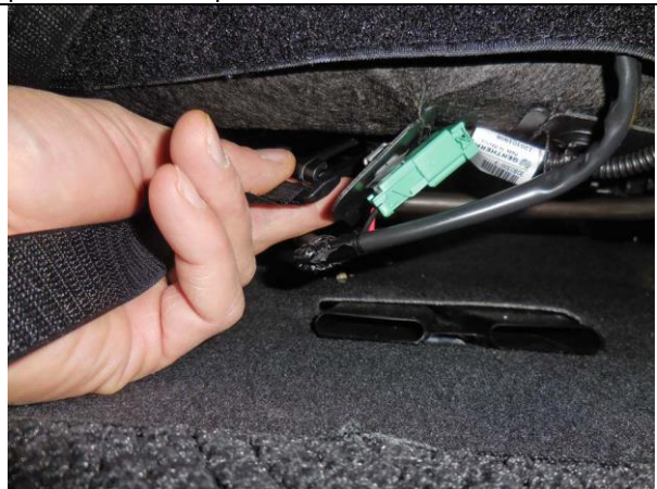
Step 18. Driver & Passenger Bottom/DB&PB: View from behind the passenger seat. Route the inside edge Velcro™ where shown by moving the electrical plug out of the way.
