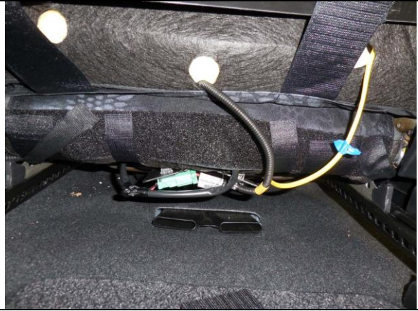
Step 26. Passenger Bottom/PB: Once connected, the Passenger side Velcro™ should look like this. The two in the center are from Steps 17-19.
