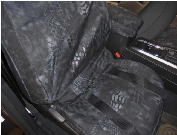
Step 27. Driver & Passenger Top/DT&PT: Slide the seat all the way forward, the slide the covers on with the extending hook Velcro™ to the front.
