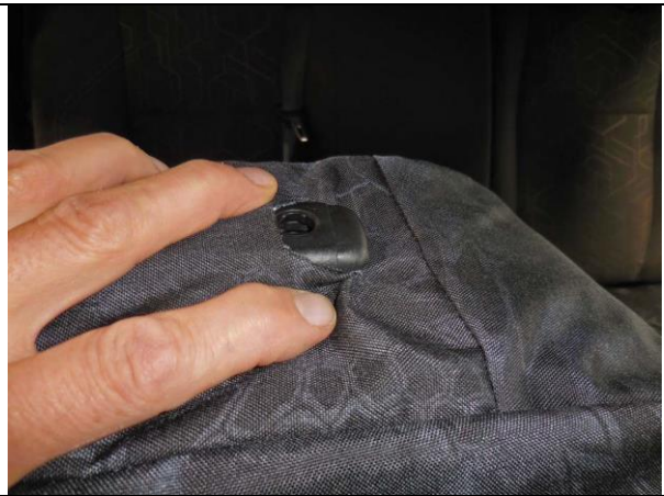
Step 28. Driver & Passenger Top/DT&PT: Tuck the fabric under the plastic for the headrests, starting with the push button release side first.
