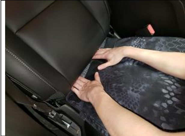
Step 5. DB/PB: Driver & Passenger Bottoms Fold the backrest forward, then tuck the back in.
