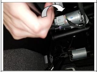
**Step 7. DB/PB: Driver & Passenger Bottoms**On the driver side, for electric seats, there is a silver motor for the seat. Make sure you feed the Velcro over the motor.
