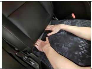
**Step 5. DB/PB: Driver & Passenger Bottoms**Take the tail end of the cover and tuck it in-between the seat top and bottom.
