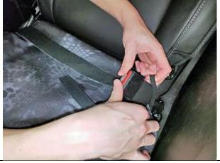
**Step 2. DB/PB: Driver & Passenger Bottoms**If your seatbelt buckle has an elastic strap around it, remove the strap.
