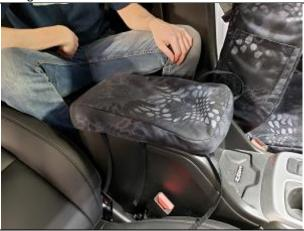
**Step 20. L: Lid**Disconnect all the Velcro and place the cover on with the "L" toward the back of the cab.
