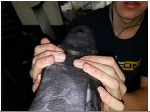
**Step 14. DT & PT: Driver & Passenger Tops**Once the cover is pulled down, the plastic headrest slots can be slipped through.
