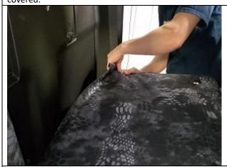
**Step 19. DT & PT: Driver & Passenger Tops**Take the back flap, pull it down tight, and paste it to the fuzz as well.
