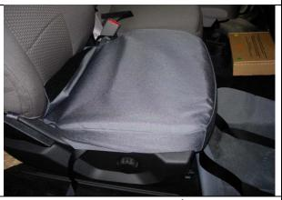
Step 6. Driver & Passenger Bottom/DB&PB: Remove the plastic buckles from the back edge of the seat cover and slide the covers on with the extending hook Velcro™ to the front.
