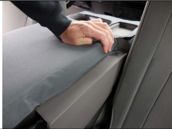
Step 27. Armrest/A: Lastly, tuck the fabric behind the plastic as shown.
