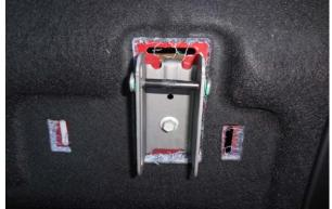
Step 12. Driver & Passenger Top/DT&PT: Make sure the driver side back wall catch is positioned where shown. Lift the driver side seat bottom up all the way and push the backrest in until you hear it click back in. This may take a few tries.
