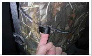
**Step 10. Passenger Top/PT:**Feed the nylon seat release trap through the provided opening.
