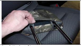
**Step 2. Headrests/H:**Form the cover to the headrest by lining up the seams of the cover to the seams on the headrest, they should closely match.
