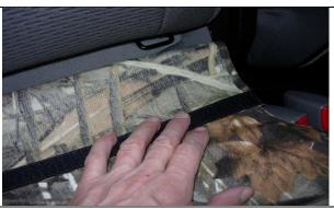
Step 4. Driver & Passenger Bottoms/DB&PB: Slide the seat covers on with the letters DB & PB to the top. Line up the seams of the seat cover to the seams of the seat, and line up the opening for the seat release latch as shown.
