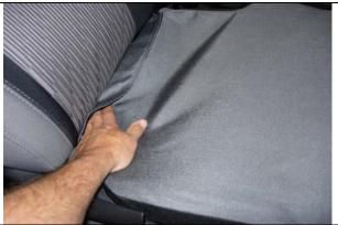
Step 7. Driver & Passenger Bottom/DB&PB: Tuck the back edge of the seat cover into the seat. From behind the seat, pull the seat cover back to conform the front of the seat cover to the seat.
