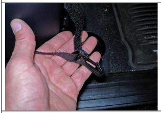
Step 21. Driver & Passenger Bottom/DB&PB: View from the front outside corner of the passenger seat bottom. The driver seat cover also has this buckle. Disconnect the Velcro™ on the buckle.
