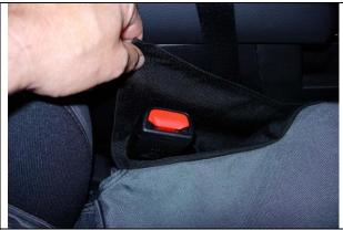
**Step 5. Driver & Passenger Bottom/DB&PB:** Tuck the seat belt though the provided opening.
