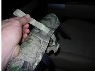
**Step 30. Middle Bottom/MB:**Tilt the seat bottom up and feed the release strap through the provided opening in back.
