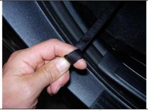
Step 14. Driver & Passenger Bottom/DB&PB: Curl the Velcro™ around your finger two times.
