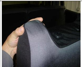
**Step 25. Driver & Passenger Top/DT&PT:**Form the top corners of the seat cover to the seat by pulling down on the bottom edge of the seat cover.
