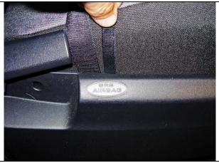
Step 12. Driver & Passenger Bottom/DB&PB: As in Step 9, fold the outside edge Velcro™ in half lengthwise and slide it behind the plastic cowling where shown.
