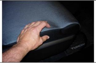
**Step 8. Driver & Passenger Bottom/DB&PB:**Line up the seams of the seat cover to the seams of the seat, they should match closely.
