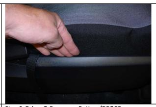
Step 6. Driver & Passenger Bottom/DB&PB: Tuck the seat cover behind the plastic cowling on the outside edge, but leave the Velcro™ out.
