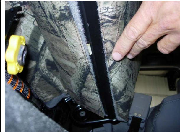
Step 19. Driver & Passenger Bottoms/DB&PB: Pull the bottom side of the seat cover down, and press the Velcro™ to the carpet on the seat.
